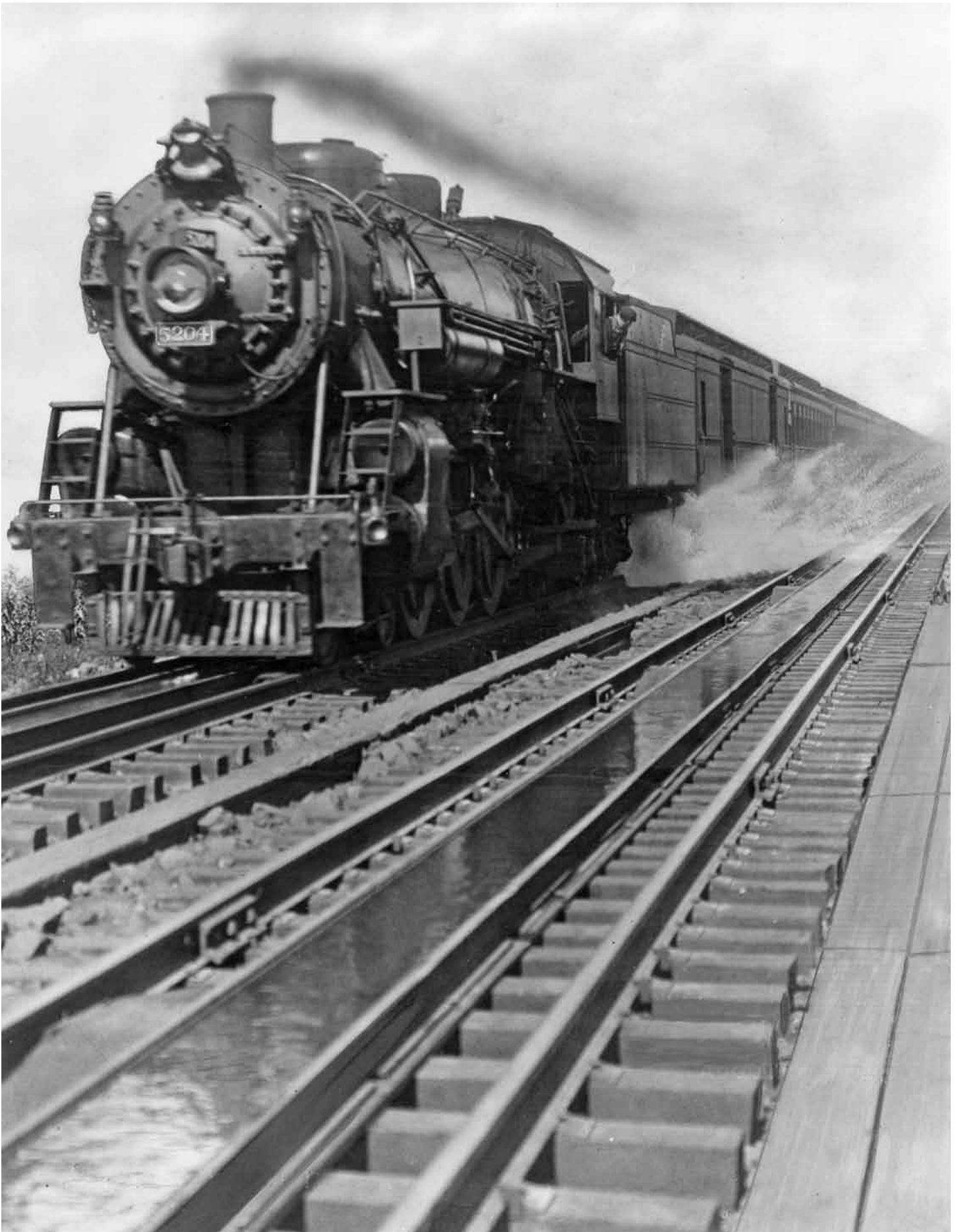
On the class P-5 Pacifics, the scoop control was located on the fireman's side. Westbound at Swan Creek in the early 1920s, the fireman of 5204 checks his work in this enlarged cropping of the photograph on page 3.
