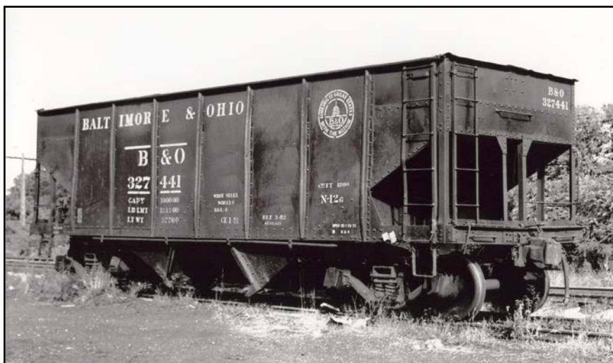
327441 Location and photographer not indicated, September 19, 1951, Bob's Photos. Right side and A end; good view of outside air line and coupler cut lever. Built 3/1923, American Car & Foundry
