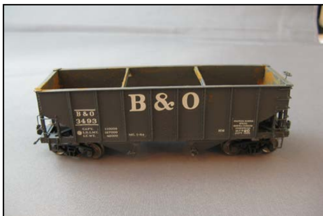
B&O 3493 "CNJ" Funaro & Camerlengo kit; F&C decals. One of numerous groups leased over the years from CNJ. Note unusual 9 panel/8 posts vs. more typical 8/7 arrangement.
