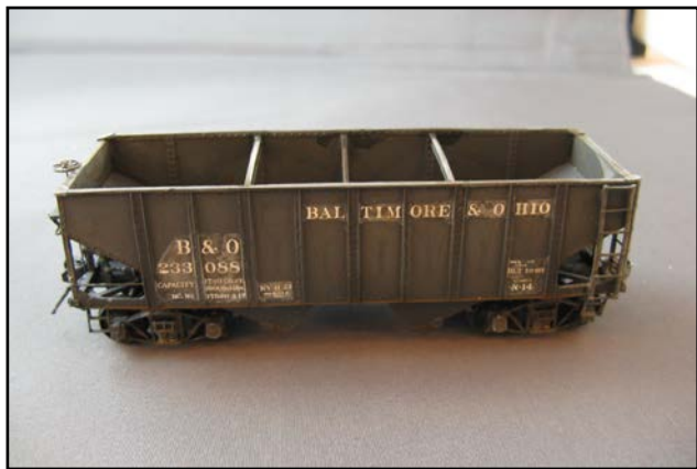
B&O 233088; N-14 Westernfield PRR GLb kit. Built 1903 for Jamison Coal Co. Very close to PRR GLb design (structural steel as opposed to pressed steel components). To B&O in 1906. Cinder service by 1929. Westernfield decals.
