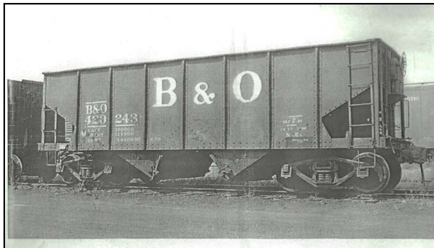
420243 Part of last lot of N-12g's built 2/1924, Pressed Steel Car. Photographer, location, date unknown, F&C Collection. Note Ajax power hand brake.
