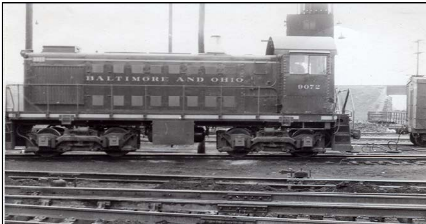
#9072, Class SA-3, Ex #528 Class DS-5a, Built Alco-GE 1943 Model S-2 1000H.P. Left side at Akron, Ohio, 1960 by Edwin C. Kirstatter. These shots were taken specifically to aid in detailing models. But, alas, I should have taken some up close shots of details, too late now.
