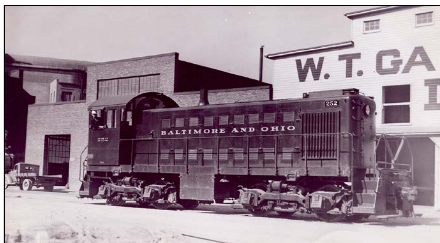
#252 Class DS-9a, built Alco-GE 1944 Model S-1 660 H.P. at unknown location and time. This is an early paint scheme--note no stripes. Credit La Mar M. Kelly. Location unknown but you might be able to find the company in a Form 6 (photo had Mr. Kelly's Elkhart, IN address on the back which is not on the B&O). There is a good chance this photo was taken on the eastern parts of the B&O as these locos were first used there before more engines were acquired and the Western regions finally got them before final dieselization happened in 1958.
