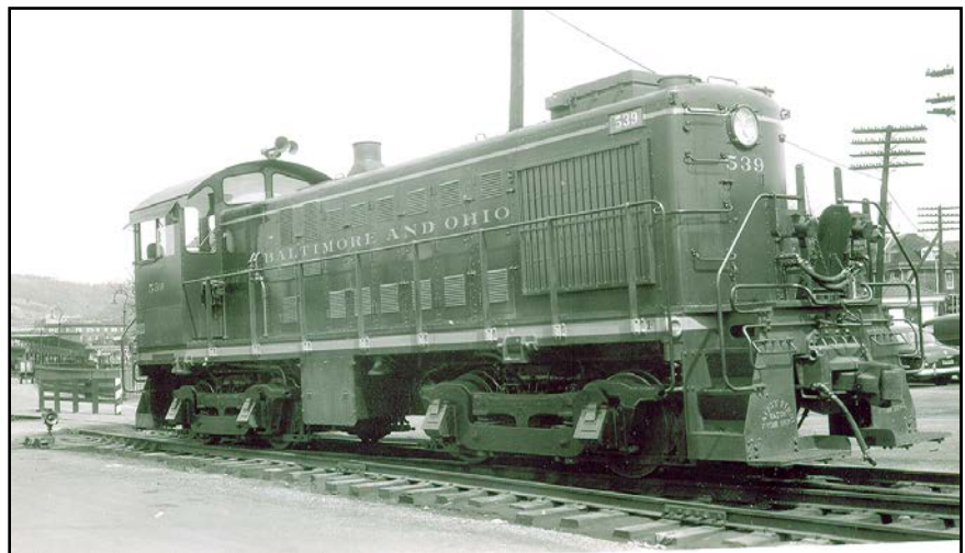
#539, Class DS-5ac, Alco-GE 1953 #80959 Model S-4 1000H.P. at Cumberland, Md. March 29, 1954. Credit Paul W. Prescott. This had MU attachments, notice no rivets on body of a late production engine. The small ‘c’ was placed after class designation that appeared on sides of cabs to show these were capable of being coupled as multiple units.
