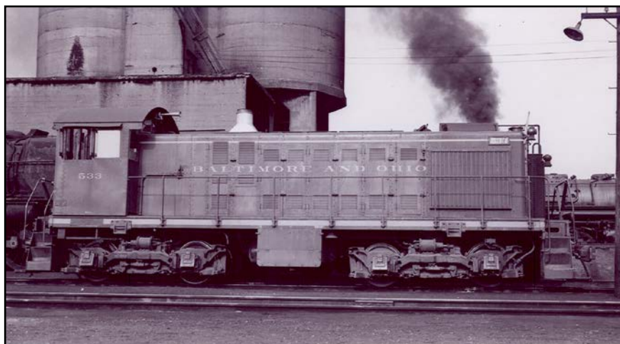
#533 Class DS-5a, built Alco-GE 1943, Model S-2 1000 H.P., at DeForest Junction, Ohio undated. Credit Paul B. Dunn. Smoke is coming from EM-1 steamer behind.
