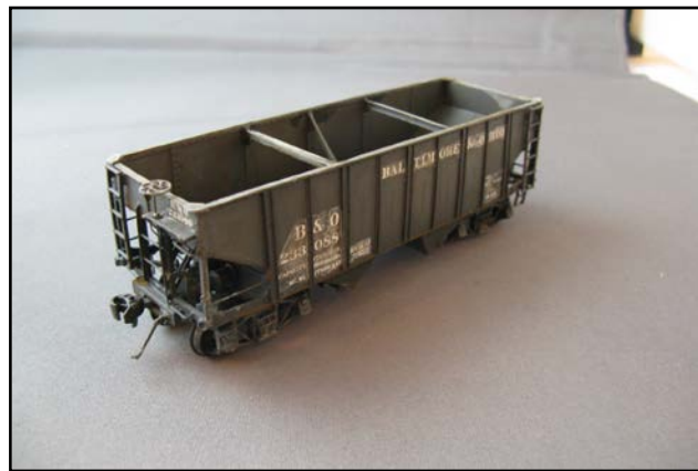
B&O 233088; N-14 Westernfield PRR GLb kit. Built 1903 for Jamison Coal Co. Very close to PRR GLb design (structural steel as opposed to pressed steel components). To B&O in 1906. Cinder service by 1929. Westernfield decals.
