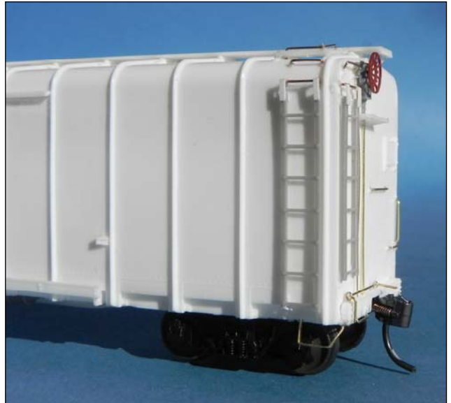
Unusual detailing on the wagontop ladders is strapping at the tops and bottoms of the stiles, and an extra straight grab on the roof curve
