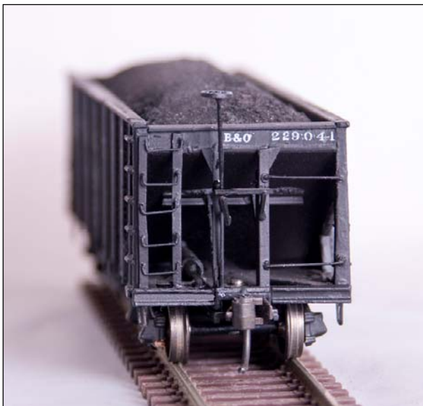
Note skinny end sheet, new end verticals and built-up "box" end sill
