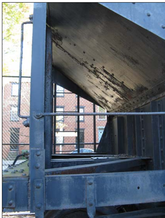
View of underside of A end. Note how the slope sheet runs at a steeper angle above the bottom edge of the side sheet
