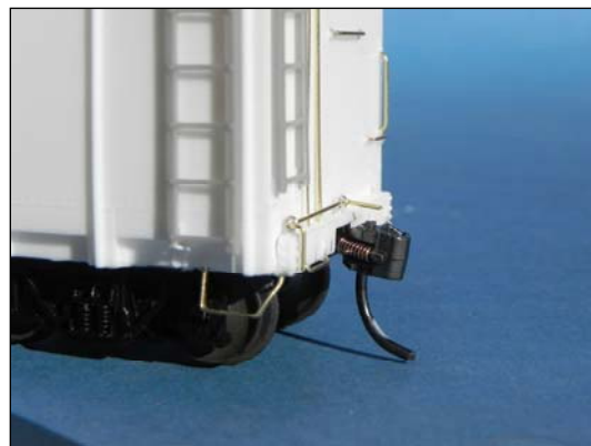
The kit provides cast resin stirrups, but a more accurate and sturdier representation can be bent from .010” x .030” flat brass bar stock.
