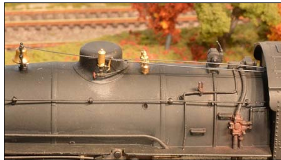
The end of the boiler walks need to angle down and finish flush with the bottom of the cab. A little resin scrap worked well for this detail.
