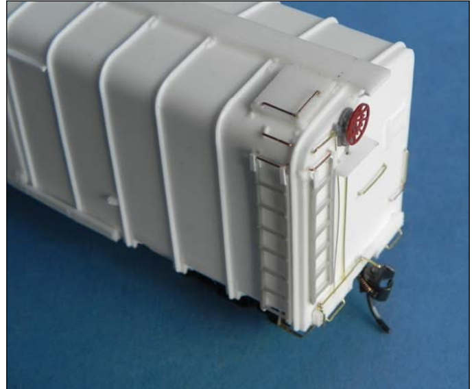
The kit provides cast resin stirrups, but a more accurate and sturdier representation can be bent from .010” x .030” flat brass bar stock.
