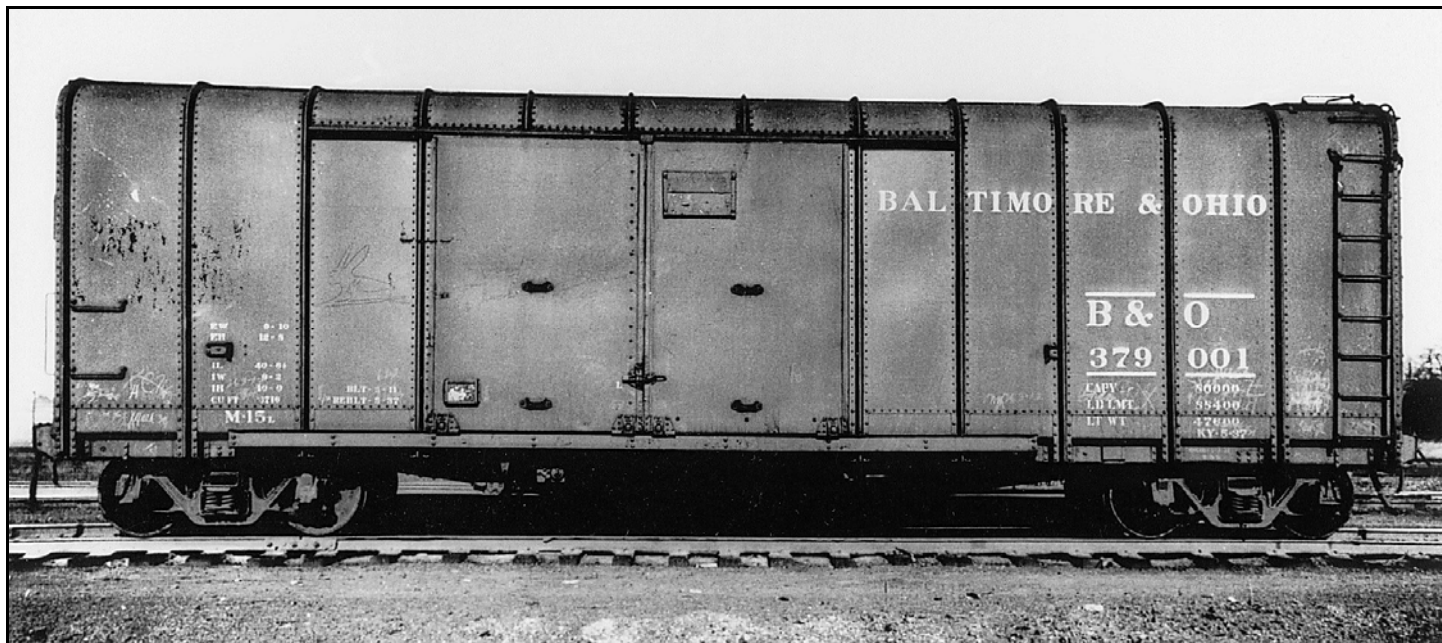
M-15L automobile car #379001 poses in its 1937 "rebuilder's photo," one of fifty (#379000-379049) rebuilt from double-sheathed M-15 boxcars of a 1910-vintage design. The original sidesill of the narrower M-15 carbody remains visible at the bottom of the M-15L side. This is the only M-15L prototype photo known to the author. Photo courtesy Martin Lofton
