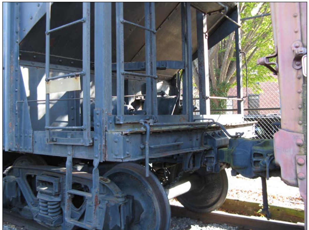
View of "box" end sill, cut lever and T-section Andrews trucks. Note the corner ladders on the side and end rather than grabs.
