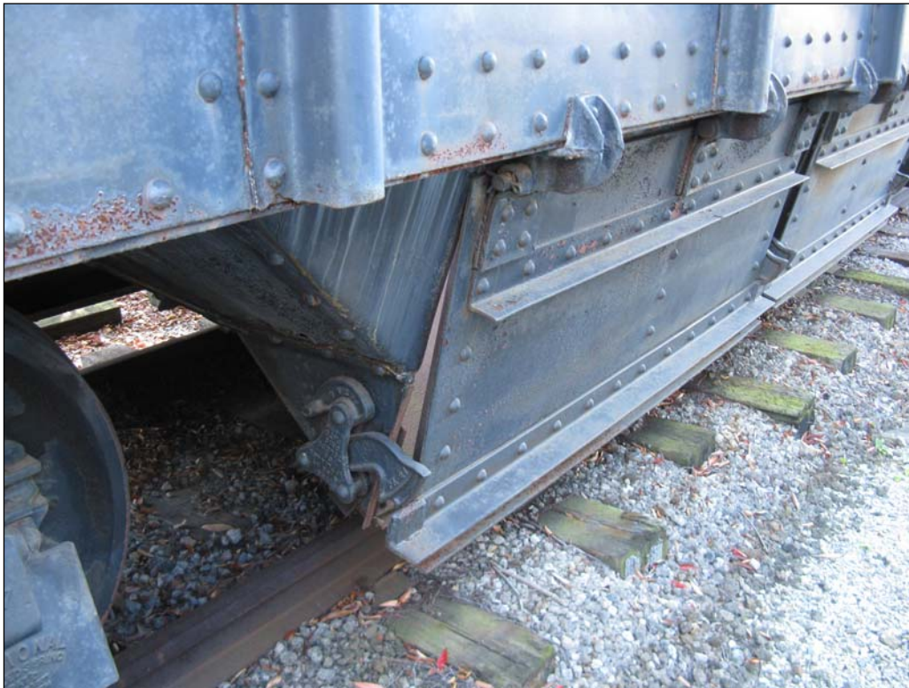
A view of the side dump doors and details of Wine door locks on the doors—Westerfield makes these latch castings.
