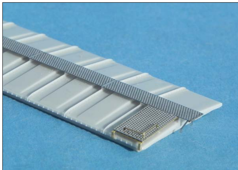
Running boards, lateral walks, and end supports complete the roof detailing.
