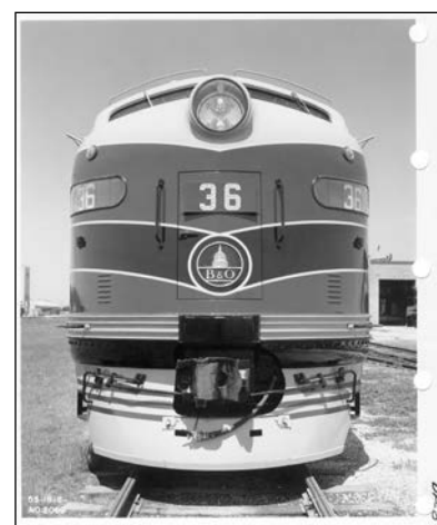
Compare the photo of E9A 36 with that of E8A 92. The differences in the headlights can be clearly seen. Photos Terry Arbogast collection.
