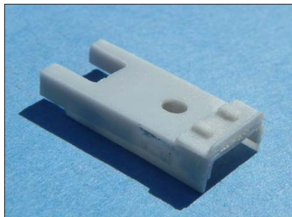
The “Duryea plate” rests atop the draft gear box, flange pointed outward.
