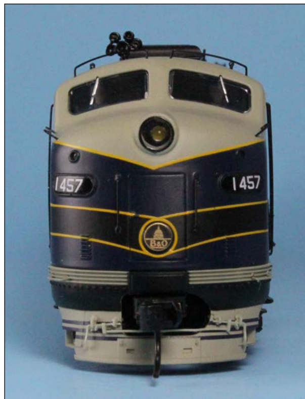
Note the coupler release rodding; Walther's supplied but modeler applied.
