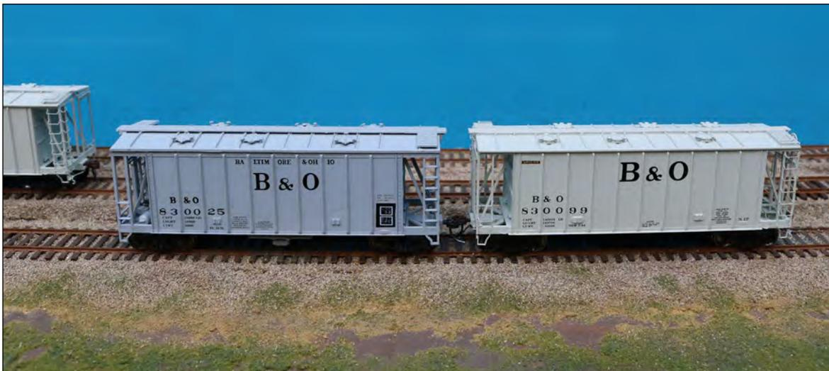
The difference in color between the Walthers model (on the left) and the Athearn models is obvious. An as-built car should have a gray closer to that of the Walthers model. The Athearn gray is probably too light for an as-built car, but weathering can be applied to make it OK for a car that has been in service for a number of years. Mike Shylanski photo.
