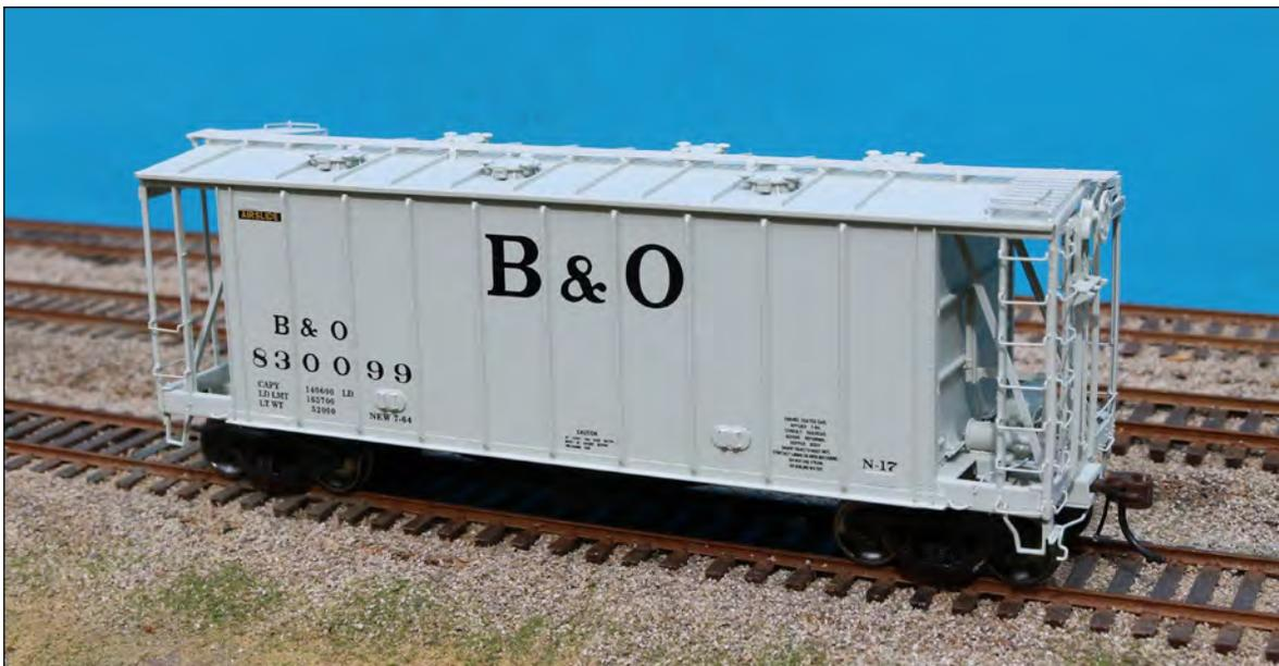
The Athearn model is neatly lettered but the gray is light. The N17 was somebody's stab at a very dirty "N47A" marking on the prototype photo of a very grungy car. Unlike the Walthers model, the Athearn model has separately applied grab irons. They look nice, but all but six of the grab irons should have been straight and not drop grab irons. Now the Walthers car, as a model of an N-47, would have benefitted from having almost all drop grab irons. Mike Shylanski photo.
