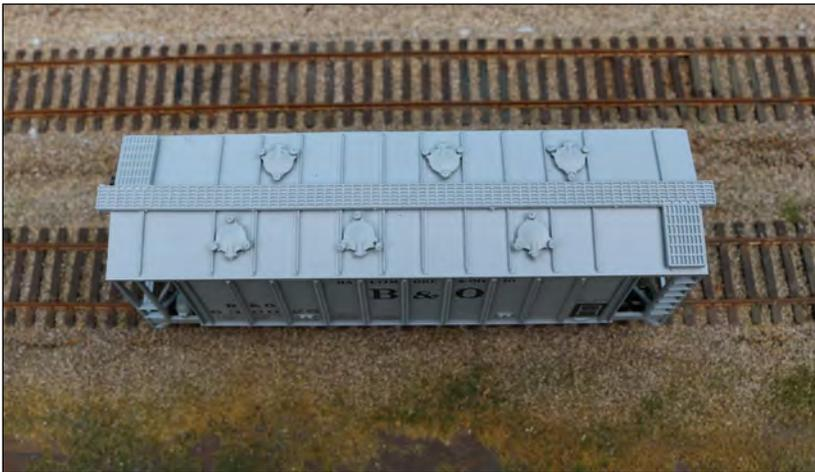
This image of the roof of the Walthers model shows that the running board (roofwalk) detail is no longer state of the art. The hatches get the idea across, but are not as nice as they could be. Mike Shylanski photo.
