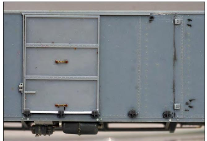
carefully shortened. The doorstops are from the Red Caboose kit. Note that the molded-on paired bolt/rivet heads under the door have been peeled off and relocated to match the cross bearers for the Duryea underframe.
