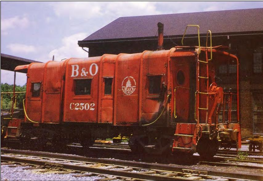
C2502 headed west at Martinsburg next to the Bridge Shop, 6/1970. Note numerous body patches and stain from stove fuel oil filler spillage on right side. It seems like a lot of modelers feel obligated to painstakingly paint the window sash green, yet you will see a lot of B&O cabs without the green, like here. John Schletzer photo scanned from *Caboose of the Baltimore & Ohio Railroad* by Robert Hubler.
