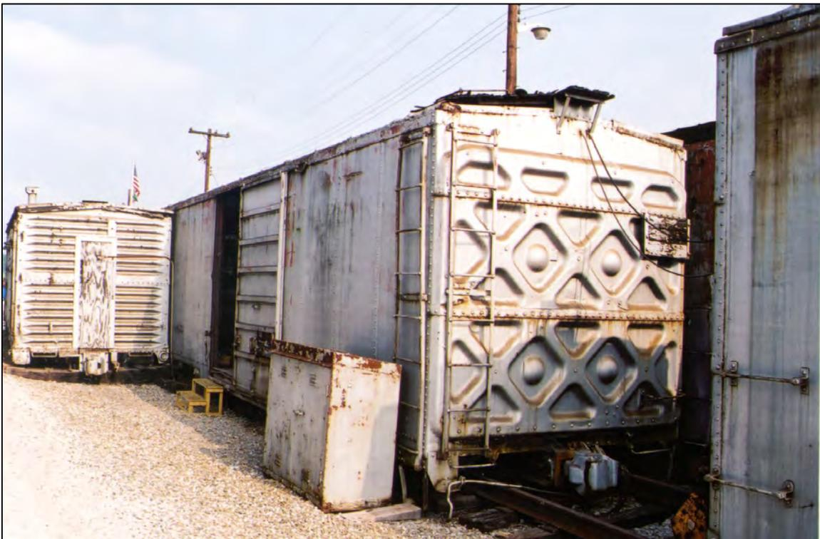
The author spotted this Deco end survivor minus its trucks at Russell, Kentucky in 2001. CSX was using whole strings of retired, 40-foot box cars to house machinery and supplies for the railroad's welded rail train. Note the partially rotted wooden running board on the roof of the grounded car. Mike Shylanski photo.
