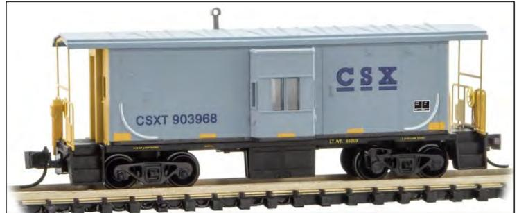
The caboose is grey with yellow ends and black lettering and runs on Bettendorf Swing Motion trucks. Even though most cabooses have been retired for decades, some still have limited use on specific areas of the CSX system. This caboose was still in service in 2014.
