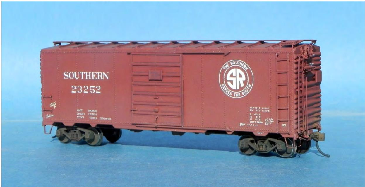
SR #23252 is a C&BT kit representing the 1944 AAR design. The prototype had 8-foot doors, represented on the model by splicing two 6-foot doors. Detail parts include a Morton running board from Yarmouth, Kadee ladders/grabs/brake wheel, and Barber S-2 trucks from Tahoe. Decals are Speedwitch. Weathering is a bit of dust with pencil highlighting.
