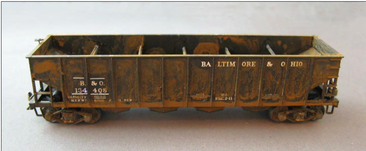
John Schletzer's W-1 from a Bowser PRR H21. The H21s in coke service originally rode on 50-ton archbar trucks, and photos of the B&O's W-1s show many on 50-ton Bettendorf T-sections as John has rendered here.
