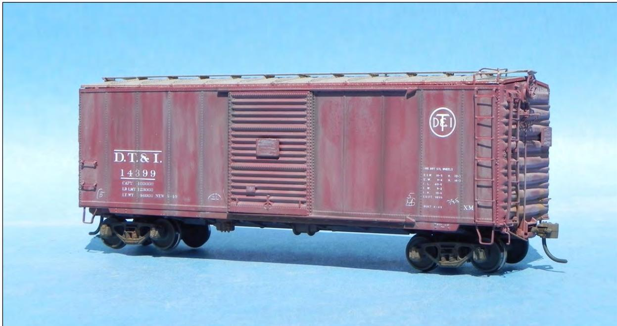
This too is a twenty plus year old kit with a lot of detail help. Continuing to clean out the three-decade stash of unbuilt styrene undec kits, Front Range kit #4070 features 10-panel riveted sides, 8-foot door, diagonal panel roof, and R-3-4 ends; a prototype near-match is DT&I's #14300-14549 series (the prototype with early improved dreadnaught ends, the model has the similar late version).
