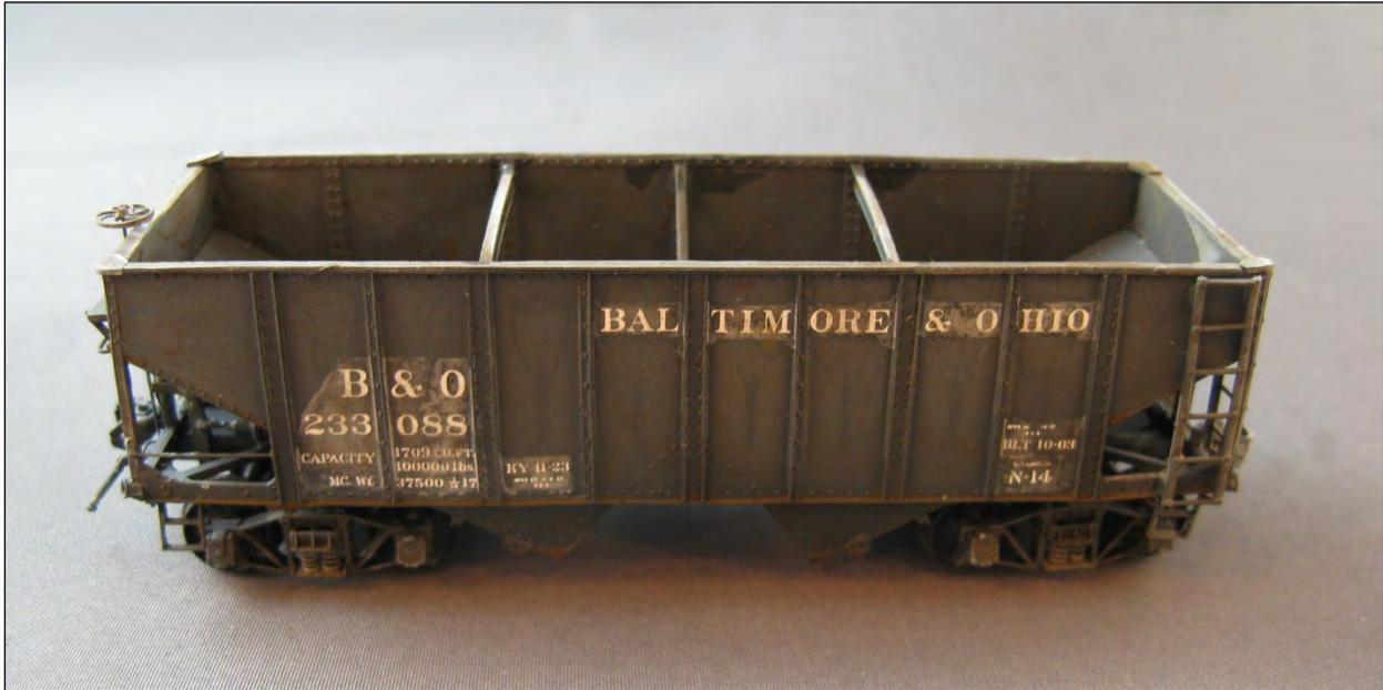
B&O N-14 No. 233088 Westerfield PRR G1b resin kit—Standard Steel Car prototype with structural shape components as opposed to pressed steel. John Schletzer collection.
