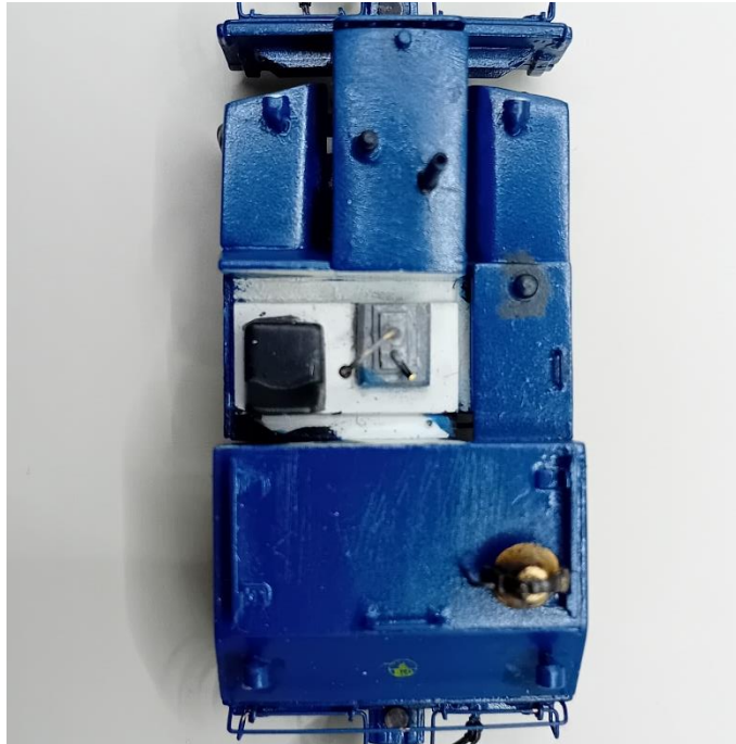
(Top view without the cab, showing the driver seat and the gearbox)
