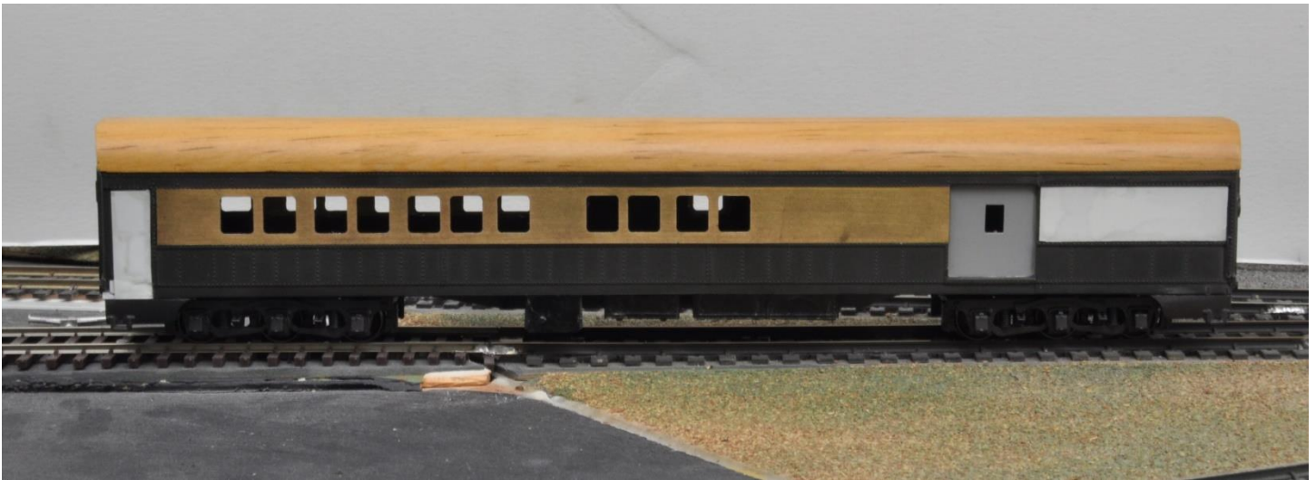
(In this view of the right side, we see the old stirrup steps have been removed from the front of the car at the right and replaced with a skirted stirrup step from a Rivarossi lightweight coach. On the left, the vestibule door has been blocked off with a .010 piece of Evergreen styrene and the stationary vestibule step has been removed. The area behind this blocked off area is now for a storage locker. Additional pieces of Evergreen styrene were also necessary to fill the void between the bottom of the door and the new skirt that now has a stirrup step.)
