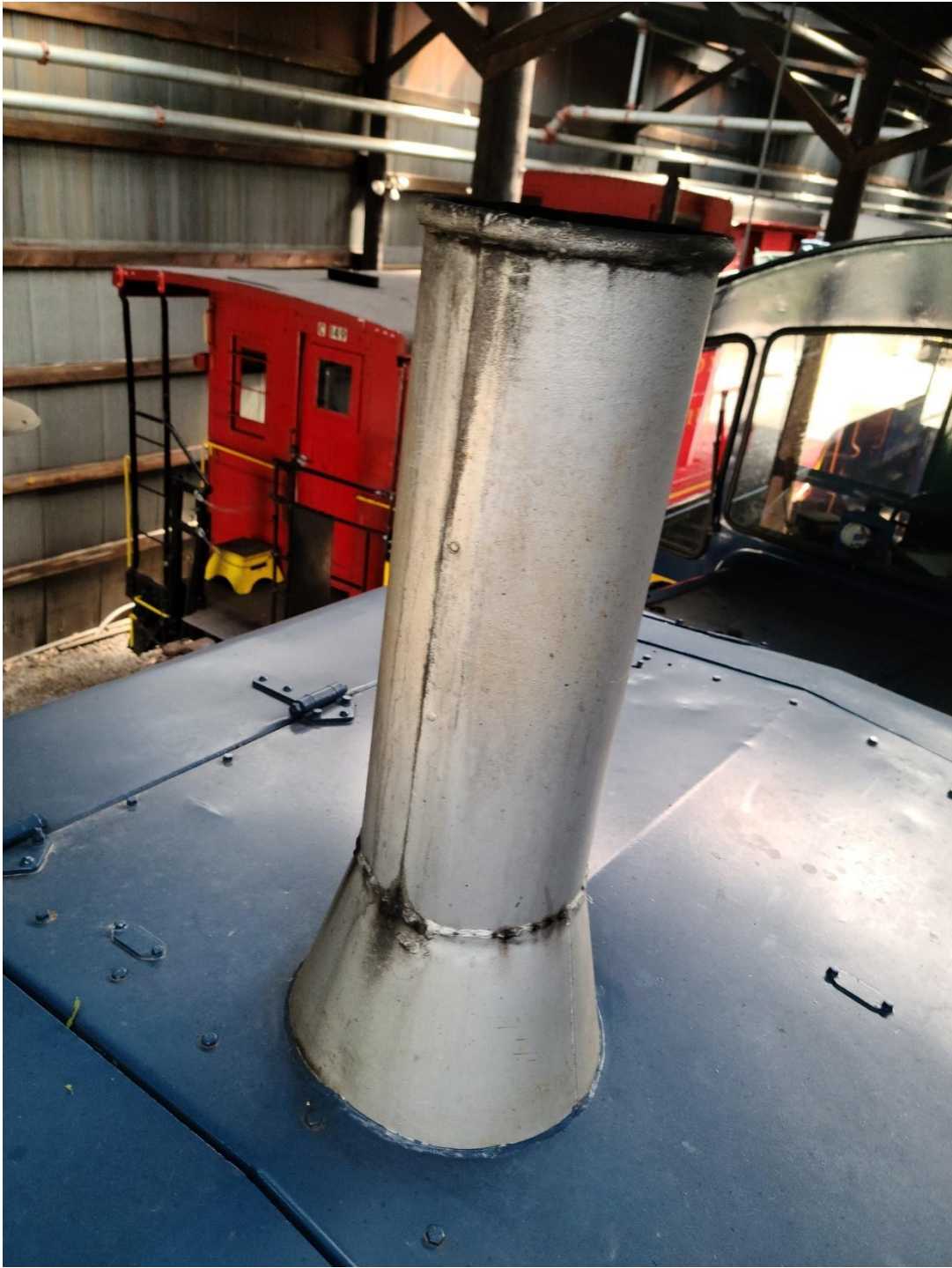
Fig 4: Photo of the stack on 8408, showing the homemade version added by the B&O to replace the unsuccessful original short stack, and the aluminum color adopted at some point in the 1950s.
