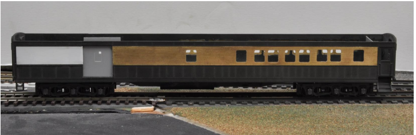
*In this view we see the left window strip installed)
