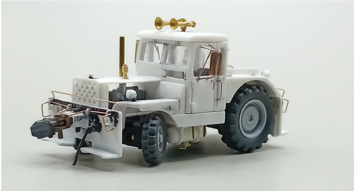
(The unpainted model with the different wheels and the steerable front axle)
