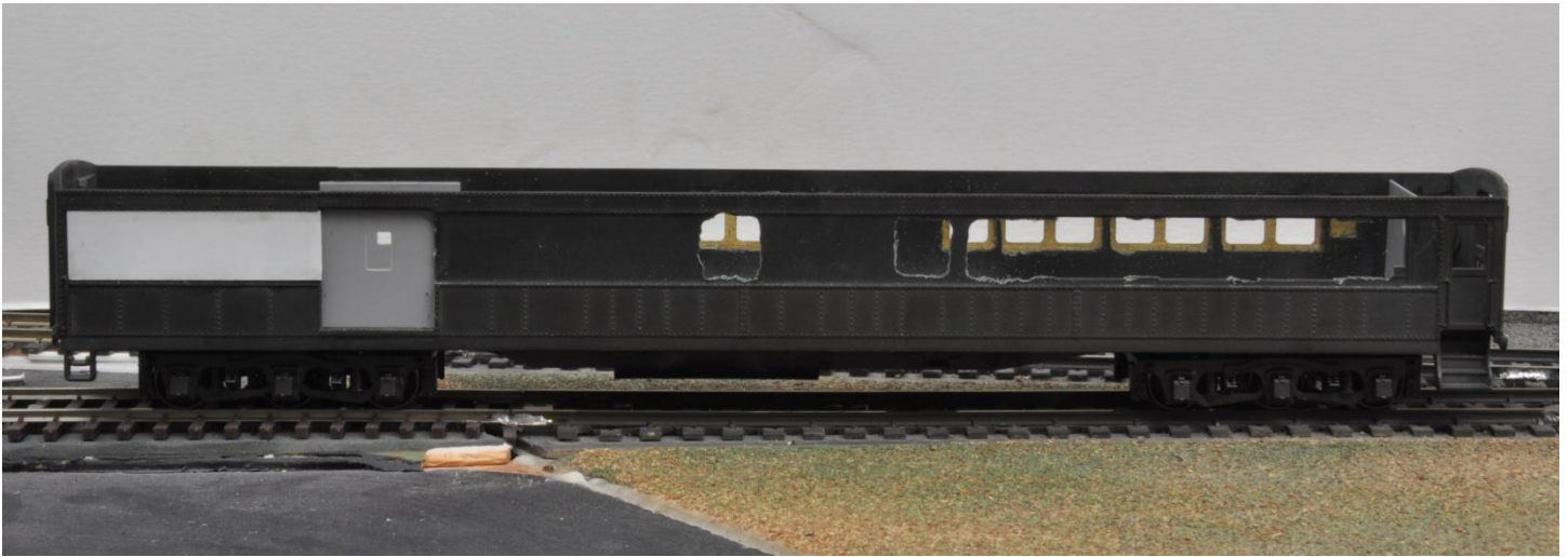
(Here we see the body after it has been cut out to accommodate the new window strip. On the back side of the interior the new window openings can be seen where eventually the new window material will be glued to the back side of the brass window strip.)
