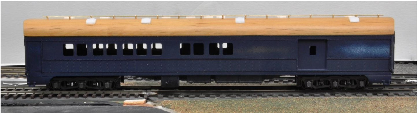
(The radio antenna has been installed. There are 16 stanchions that support the antenna, which is a .0024 brass wire. The stanchions are spaced 4.5 ft. apart. This completes the roof assembly.)
