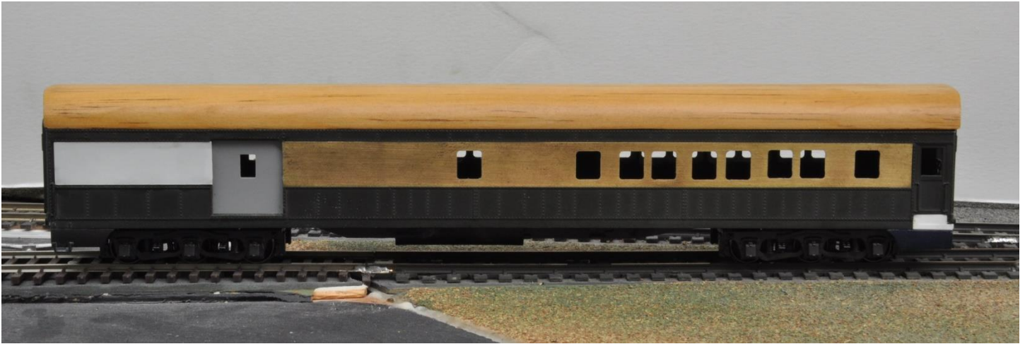
(In this left side view, the original stirrup step at the left has been removed and replaced with a skirted stirrup step that was gleaned from a lightweight Rivarossi coach. On the right, on the vestibule end is the skirt from the vestibule end of a Rivarossi lightweight coach. Note that there is no stirrup step. Behind this skirt were the folding steps. The new skirt pieces only come up to the lower edge of the body, and therefore it was necessary to use Evergreen styrene to fill the void.)
