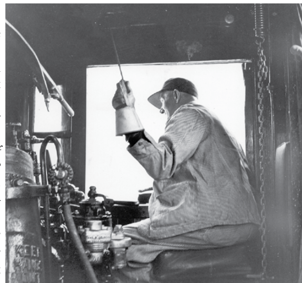
Individual engineers owned the spring-and-chain devices that hooked to the seatbox to smooth their ride.
