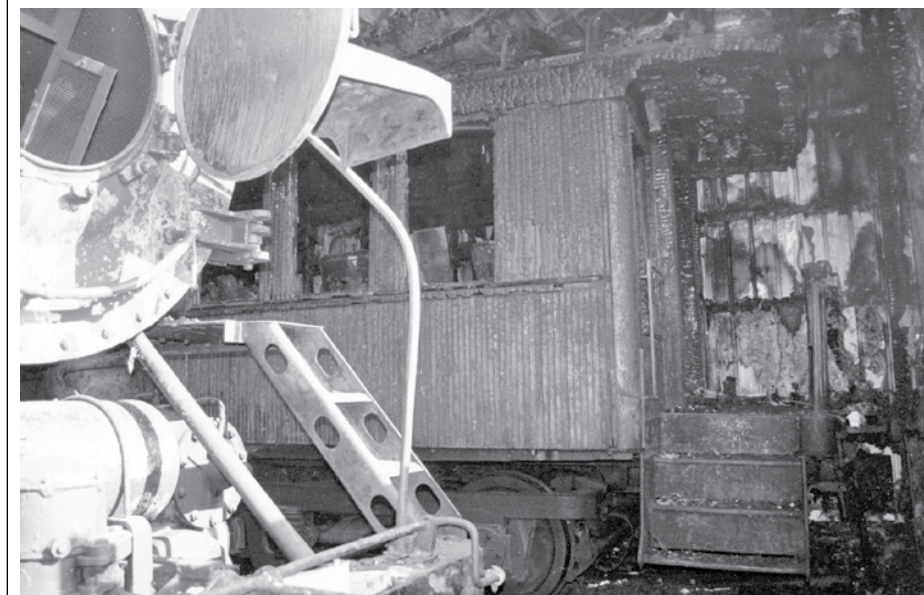
The fire that destroyed the Kane enginehouse in March did serious damage to the equipment inside. The smokebox door on the Chinese 2-8-2 was heavily oxidized and a great deal of boiler insulation was destroyed. The K&K "Presidents Car" in the background was basically so much kindling. The car was originally Delaware & Hudson Number 241. (George Kovalchick photograph)
