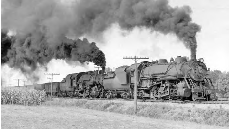
Doubleheaded Q-4s moved a lot of coal north on the former Cleveland, Lorain and Wheeling division of the B&O. These two Mikados are going through Sterling, Ohio, south of Medina, in the mid-'50s. (Herbert H. Harwood Jr. photograph)
