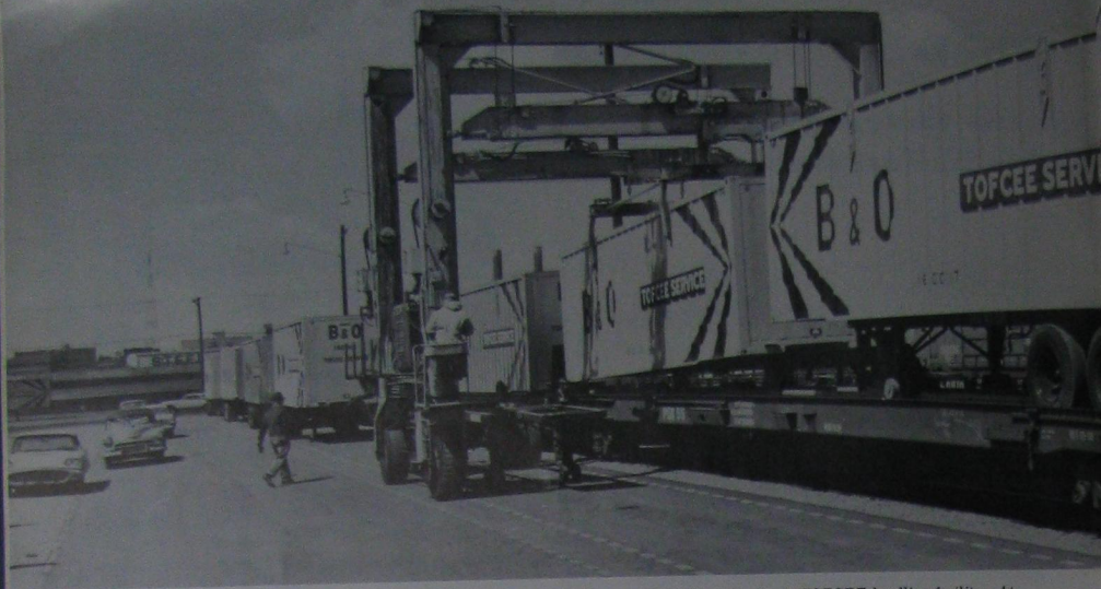
Travelift crane operator deposits demountable body onto flat car at B&O's East St. Louis TOFCEE handling facility. At present B&O has 255 demountable bodies in piggyback service, and 405 wheeled vans. An additional 100 vans are now on order
