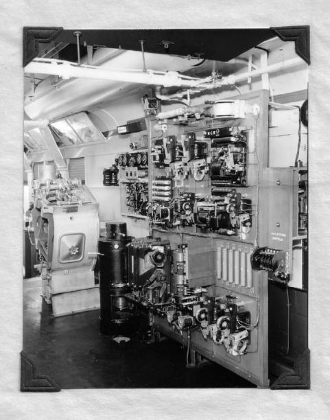
VIEW SHOWING CUT AWAY MODEL OF A 567 TYPE DIESEL ENGINE, ENGINEER'S CONTROLS AND CLASS DP-2 ELECTRICAL CONTROL PANEL
