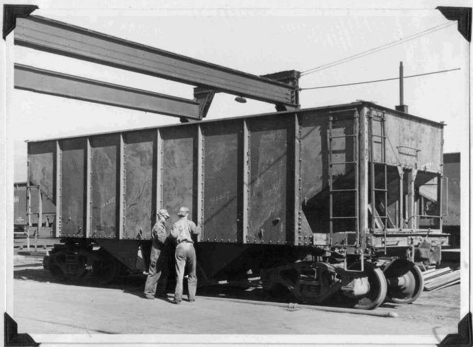
Spot "B" - After car sides are hung, cars are again placed on trucks, couplers replaced, and car moves on to Spot "C".
