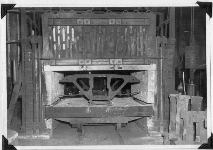
After truck frames have been welded, they are placed in furnace and annealed in accordance with provisions of the rules of the Association of American Railroads.
