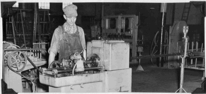
Pipe is cut to various lengths, threaded,
