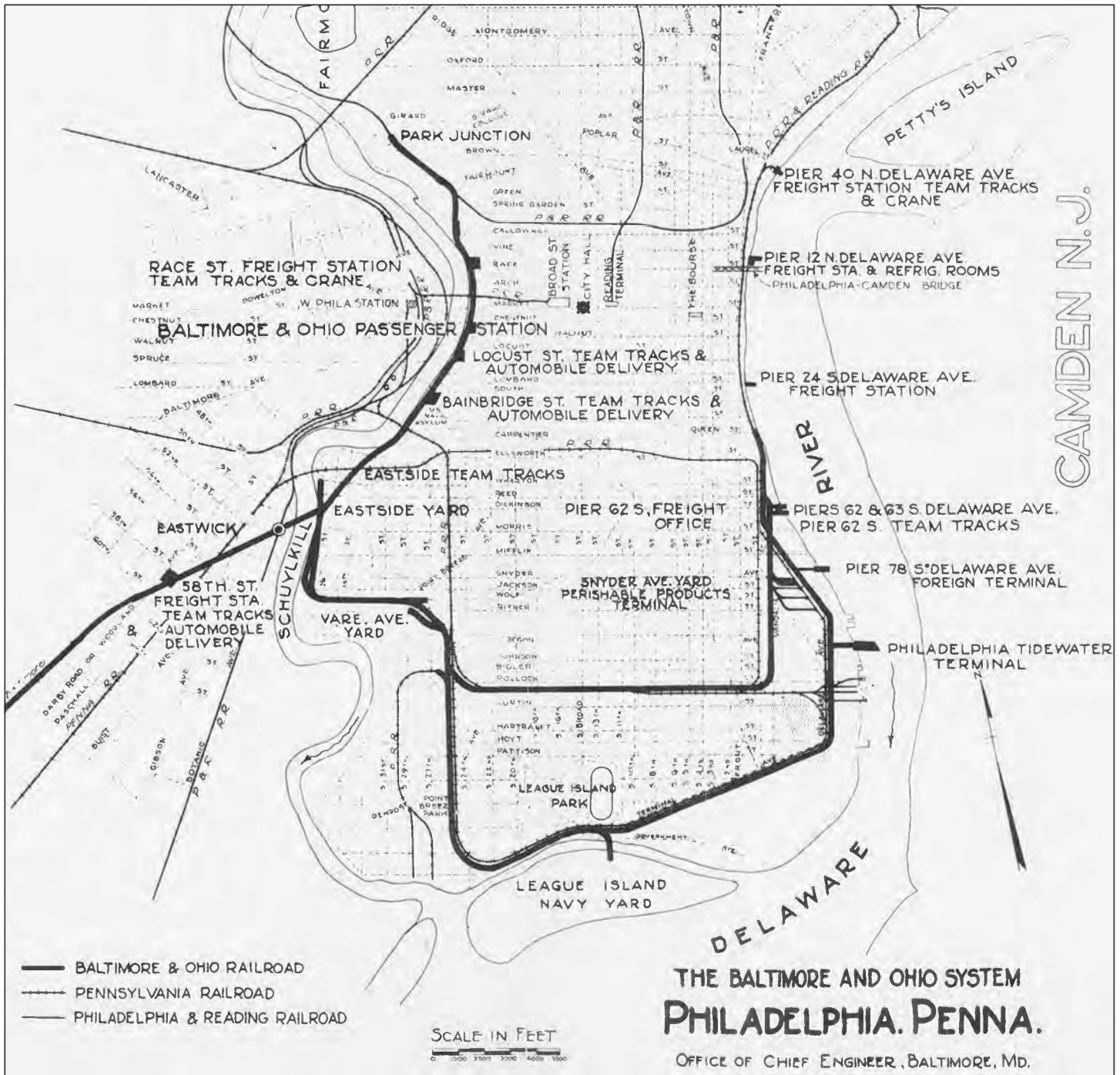
Undated map of the B&O facilities in Philadelphia, Office of Chief Engineer, Baltimore. The B&O had extensive freight facilities along the Delaware River including the Snyder Avenue Yard and the Perishable Products Terminal off Vandalia Street. (B&ORHS Archives)
