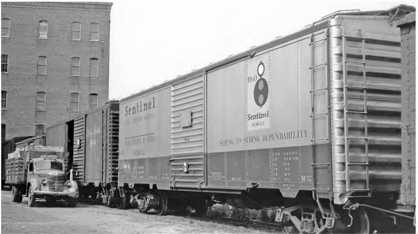
B&O M-55C 466032 built in August 1945 and last repacked on March 11, 1947, New Orleans, Louisiana, 1947.
