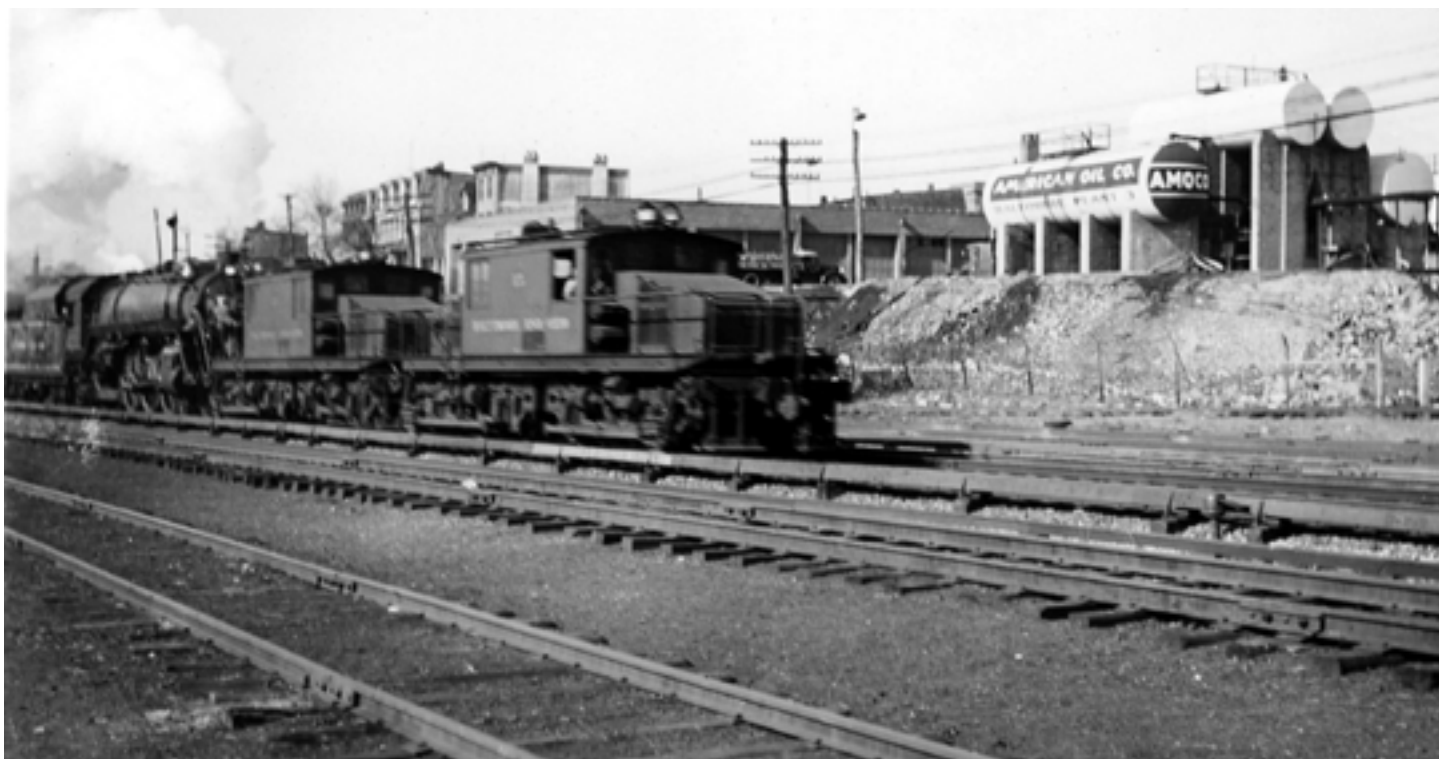
Before there were second-generation diesels, there were tunnel motors, put in service to move B&O steam-powered trains through Baltimore's Howard Street Tunnel without suffocating passengers and crew. These two were photographed at HU Tower in 1938, near the end of their service.
