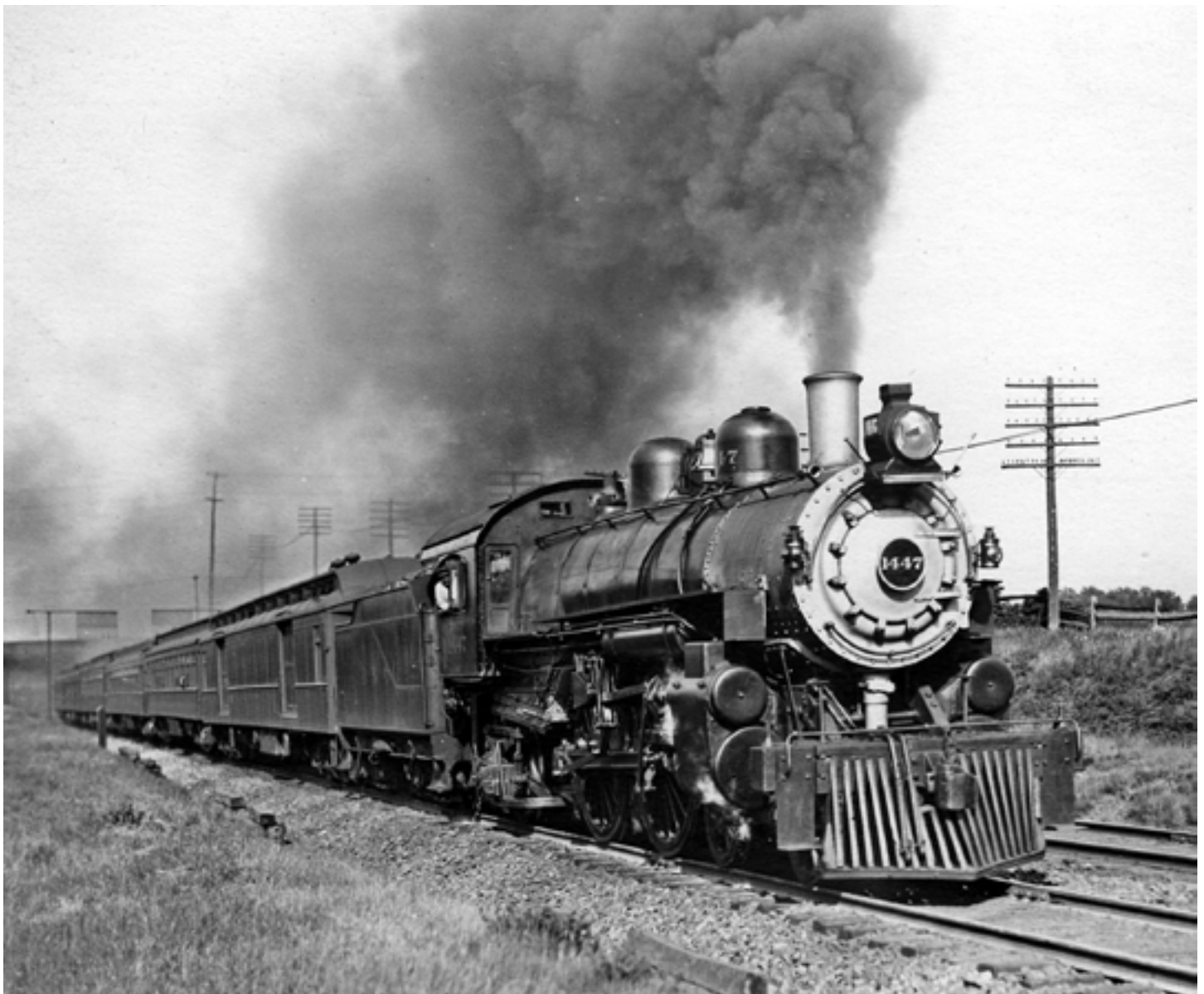
Number 1447, an A-3, pulls its train east in the Philadelphia area in this 1911 photograph. Like the 5100 pictured on page 3, this 4-4-2 is nearly new, having been built by Baldwin in May 1910.
