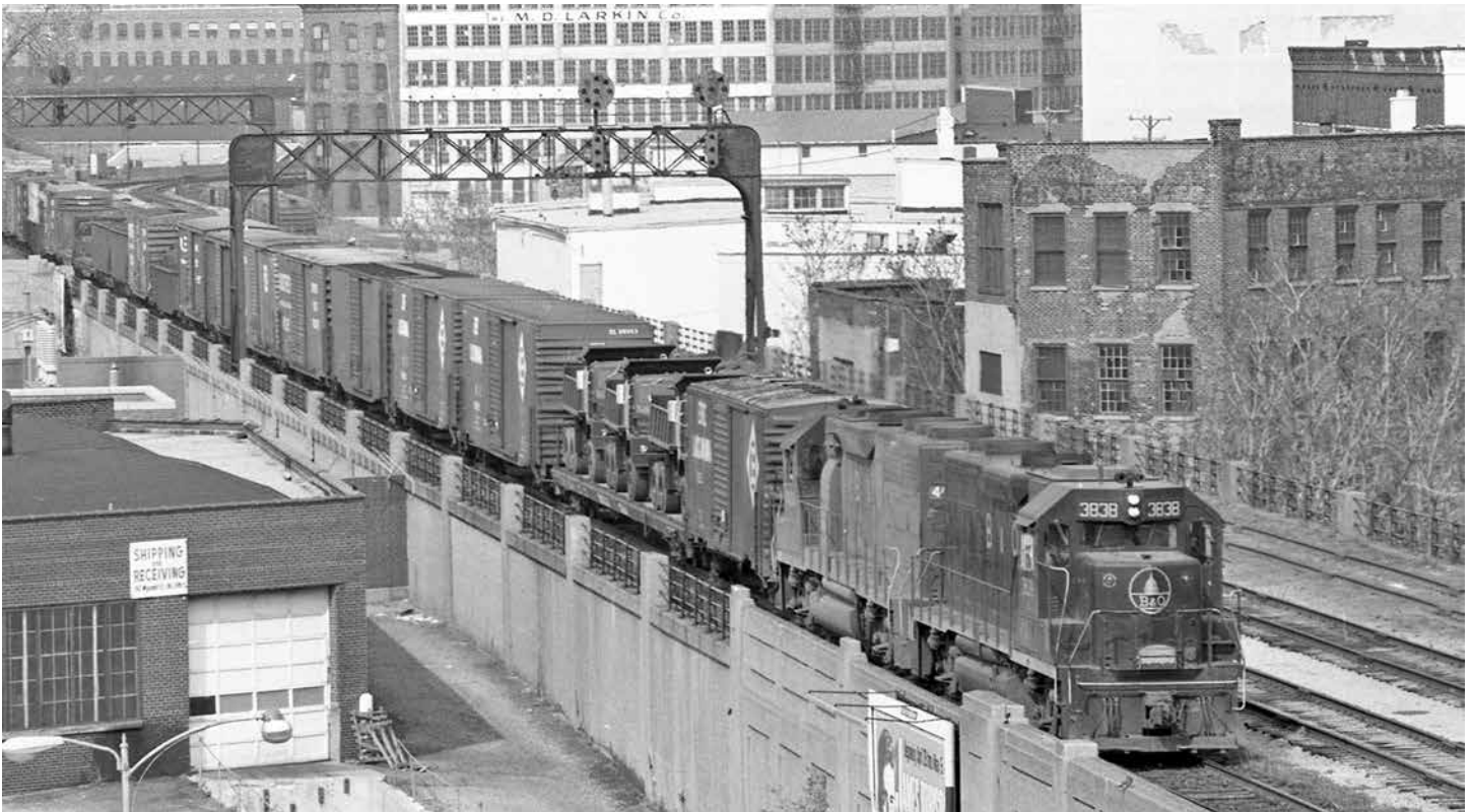
In this view from the parking garage for the Dayton Convention Center, GP38 3838 is leading a southbound train on Dayton Union Railway trackage on April 28, 1974. Dayton Union Railway was jointly and equally owned by B&O, NYC, and PRR, and it provided a route through downtown Dayton that was used by trains of all three railroads. Prior to 1931, this right-of-way was at street level, and the frequent train movements caused a great deal of traffic congestion on city streets. An elevation project, completed in 1931, eliminated all grade crossings in the downtown area. There were four tracks between Dayton Union Station and Second Street Junction, where B&O's Second Subdivision met the joint tracks. The outer tracks were for freight trains, and the middle tracks were used primarily for passenger trains.
