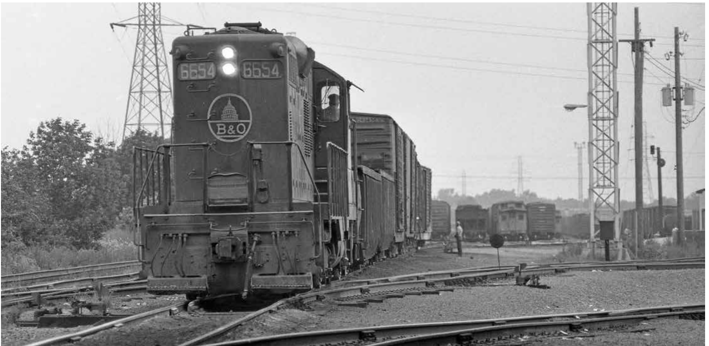
GP9 6654 was switching at the south end of Needmore Yard on July 28, 1973. Needmore became the primary yard in Dayton once an expansion project was completed in 1969. The 6654 is on the yard lead that stretched south to North Dayton Tower. To the left is the single main track (with welded rail) and the siding (with jointed rail). The six yard tracks closest to the main and siding are the original Needmore Yard tracks. Eleven more tracks were added in the expansion project. The tracks curving to the right go to the car shop and the engine servicing area
