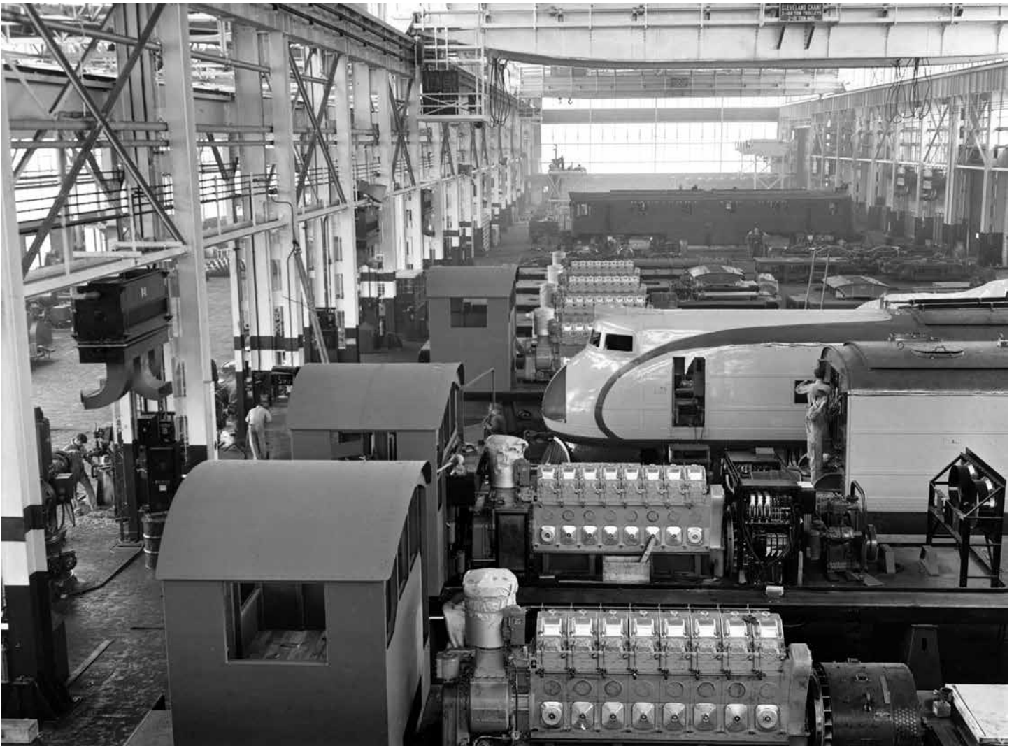
B&O 50 Class AA at EMC with new shovel nose in background; UP M10002 in foreground. Since 50 was delivered in 1935, the shovel nose was applied at Mt. Clare in 1936, and M10002 was built in 1936, 50 was back at EMC in 1936 to address some teething problems. Per Jim Mischke, 50 had both electrical problems and truck mechanical problems. (Collection of B&ORRHS)
