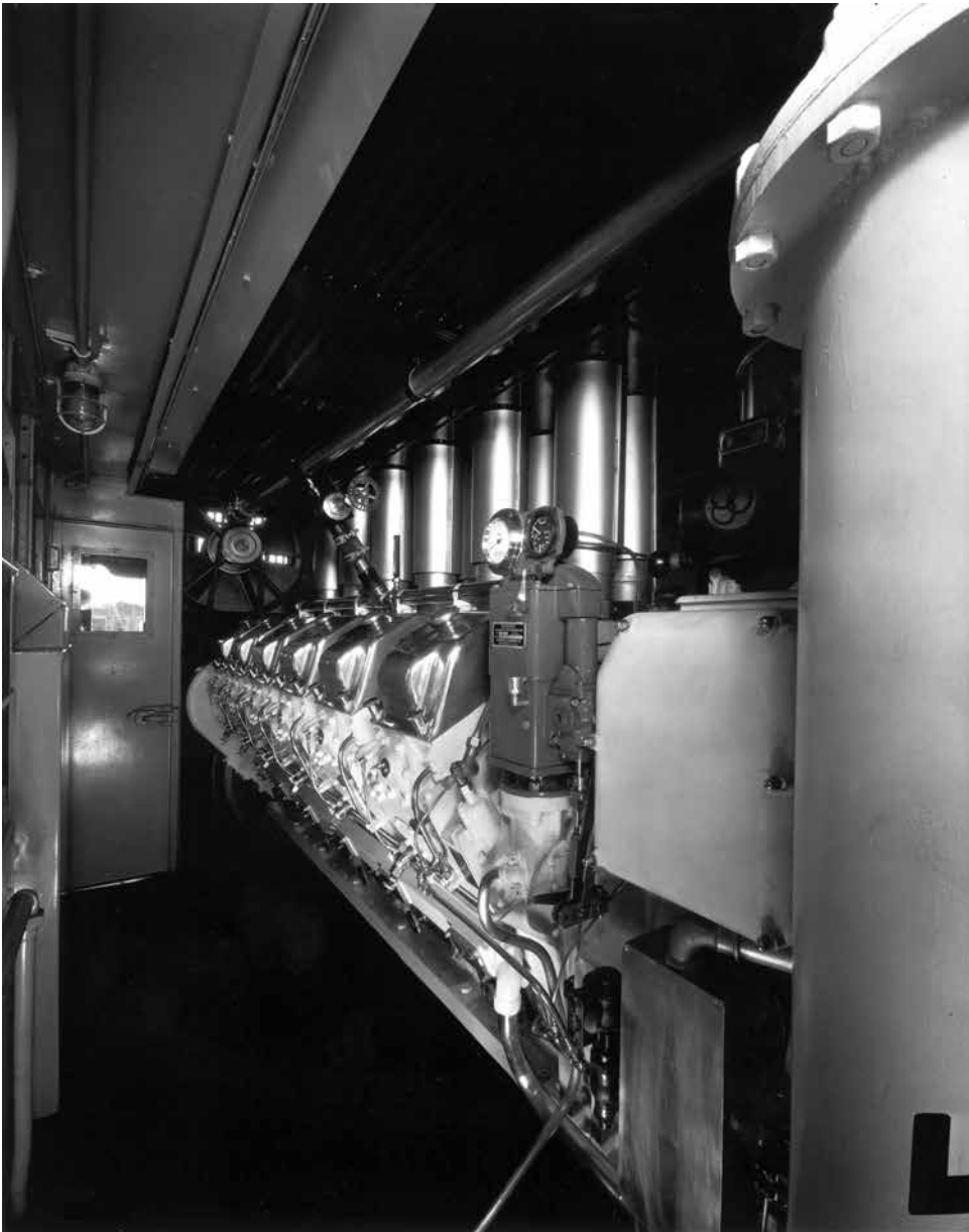
B&O 50 Class AA interior showing Winton Engine. (Collection of B&ORRHS)
