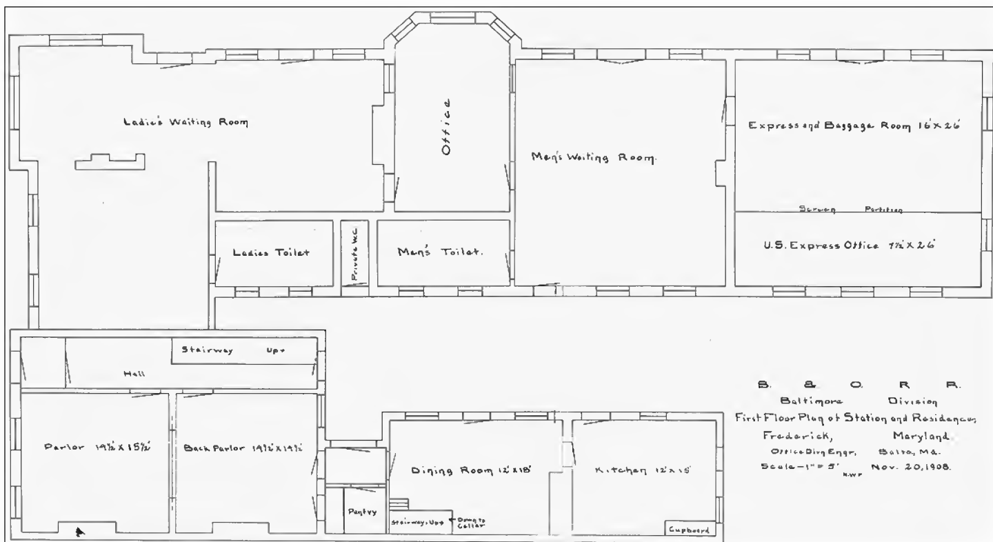
Floor plan of the first floor of the Frederick Passenger Station from a November 1908 B&O drawing. The ladies and men's waiting rooms opened to the track in All Saints Street at the top. (B&O RHS Archives)
