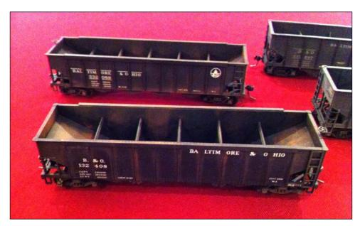
W-1 hopper by Geroen Gerritsen. He upgraded a Bowser PRR H21 with "old style" doors by adding top reinforcing chord, modifying end beams and replacing the cast-on grabs with ladders. (AY)
