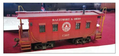
I-1 No. 307 by Geroen Gerritsen. Started with Pro-Custom Hobbies (Quality Craft) kit; used only the basic wood frame and most castings from kit except window castings. Made sides, ends and roof from styrene. Railings, ladders smoke jack were all built up from brass. Window sashes came from a Pacific Mountain Shops kit. (CS)
