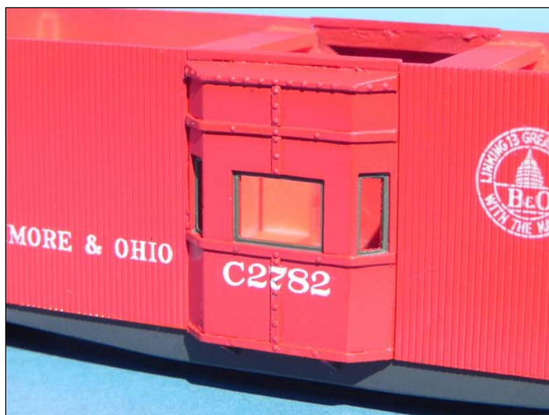
A scrap of decal painted Pullman Green and cut into narrow strips makes it easy to achieve a sharp edge between the green window sash and the red carbody. A few licks of green will touch up the inner edges of the sash.
