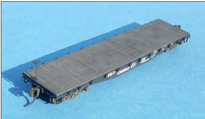
Some highlighting with Prismacolor pencils adds subtle color differences between individual boards
