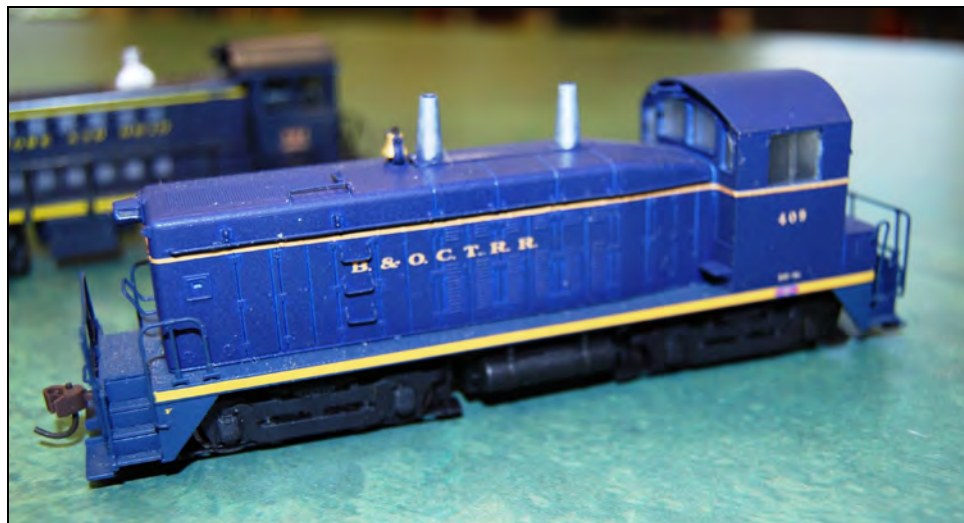
BOCT 409 EMD NW-2 - Broadway Limited model repainted Scalecoat II B&O Royal Blue and lettered with Ed Sauers decals. The factory supplied decoder was defective so it was replaced with LokSound Select Micro decoder installed. Project done by Bill Hanley for Henry Freeman. (The BLI NW-2 is a nice unit—great reverb; I bought one not long after they were issued and my lighting effects were quirky. The company offered to fix it if I sent it to them at my expense. I waited, and the decoder "righted itself." Do these things have souls? Possessed? JT)
