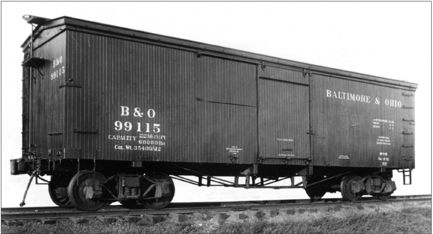
M-8b 99115 shown after a steel centersill was installed at the Ralston Steel Car Company in 1912. (RSC Negative 252-1200)
