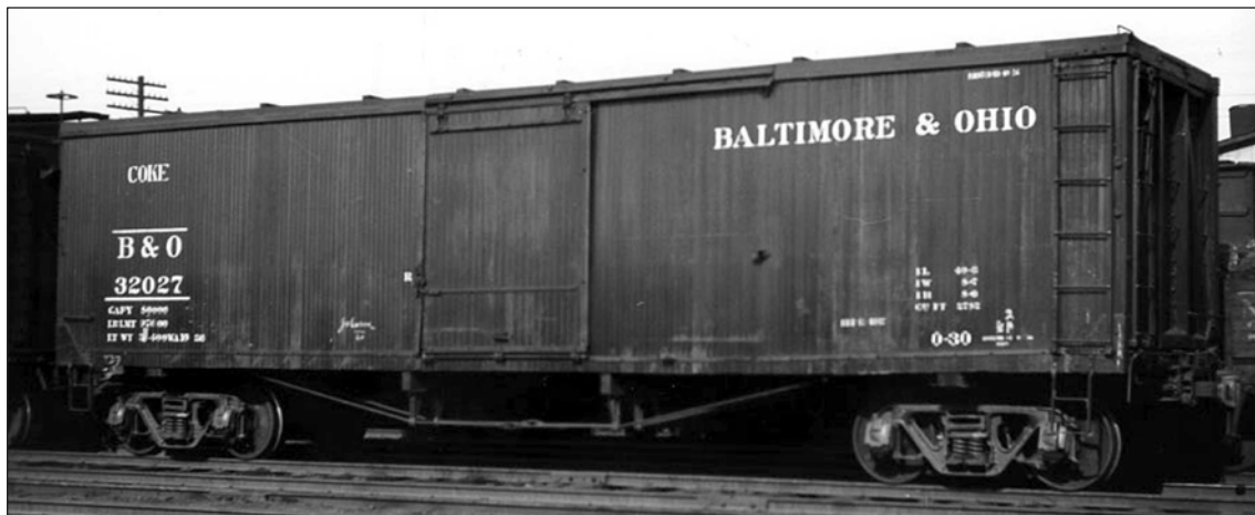
Former M-18 in 1950s with roof removed for coke service and reclassified as O-39b. The car in this photo is mis-stenciled. (Jay Williams photo collection)
