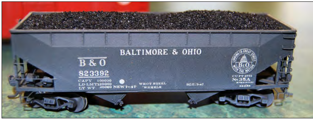
N-35a 823392 - Heavily modified Athearn kit (See March 1991 issue of Model Railroader ). Bill was on the "clinic circuit" in the early 1990s showing how he upgraded the Athearn hoppers with grabs, air piping and other details. This was on an early wave of the "Prototype Modeling Movement," and long before Tangent, ExactRail, Proto 2000, etc. Bill's upgrade process in some circles became referred to as "Hanleyizing". JT)
