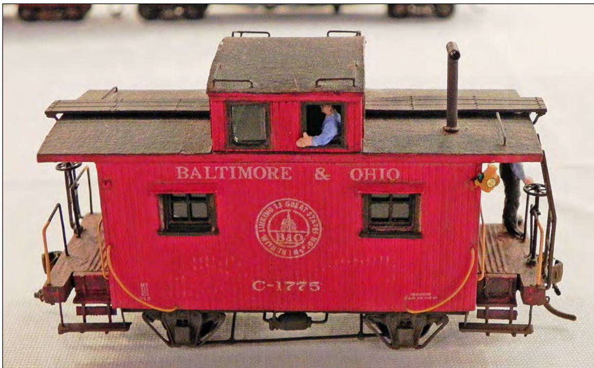
Class I-11 four-wheel bobber #C-1775 was kitbashed from a Bachmann model. The prototype was retired in 1956 and is preserved at the B&O Museum.
