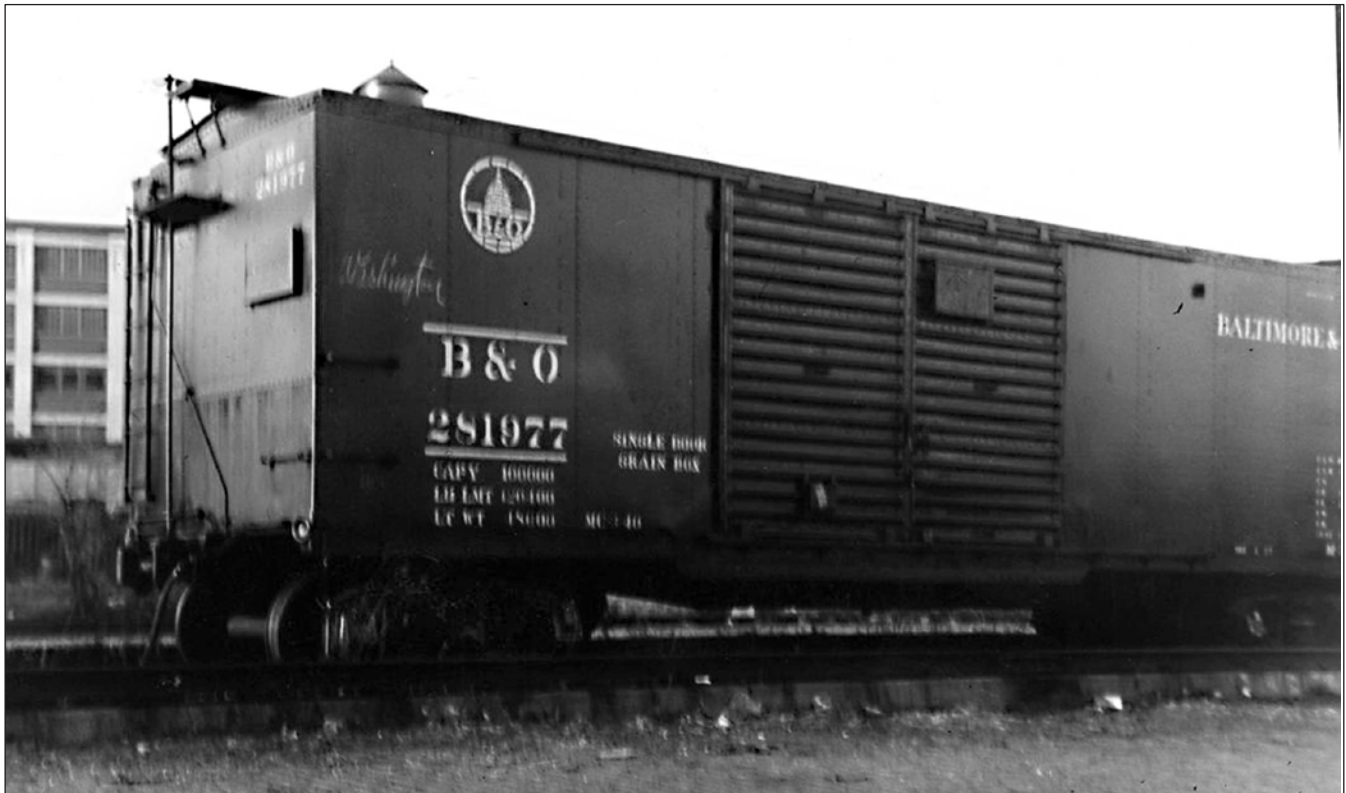
M-27 281977 in 1946-47. The car has had some modifications since being built as there is a full extra door but the car is stenciled as a single door car for grain service
