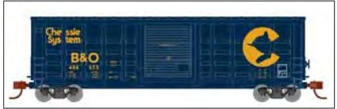
On the model, in addition to the distinctive indentations on the body of the waffle car, spotting features include outside posts, non-terminating corrugated ends, and a slightly peaked roof. No Chessie System class is claimed or legible on released art. <http://www.athearn.com/Products/Default.aspx?ProdID=ATH25374>
