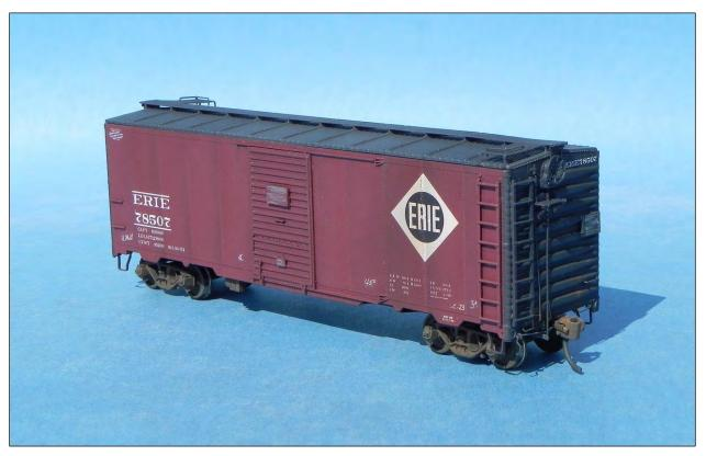
Erie boxcar #78507 is an IMWX kit representing the 1937 AAR design. The kit roof was replaced with a Viking roof, a feature of the Erie prototype. Added detail parts include Tichy 8/8 ladders, an Apex running board from Yarmouth, a Kadee Ajax brake wheel, and National Type B trucks from Proto 2000. The black roof and ends were Erie features; decals are Speedwitch Media.
