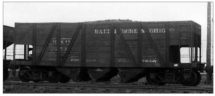
The N-16 and N-16a cars were distinctive, as you see above. They were wood construction with steel underframes and truss members following a Seley design. The B&O was rebuilding these cars in the mid-1920s with steel hoppers, steel ends and open sides under the slope sheets at the end sills.
