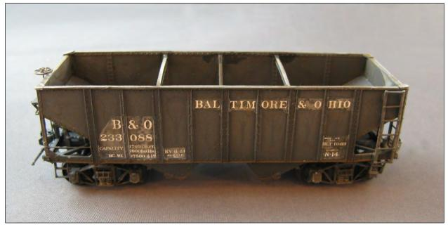
B&O N-14 No. 233088 Westerfield PRR Glb resin kit—Standard Steel Car prototype with structural shape components as opposed to pressed steel. John Schletzer collection.
