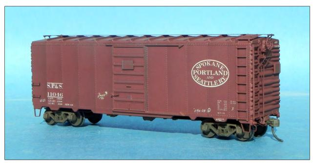
SP&S #11046 is also a C&BT kit representing the 1944 AAR design. Detail parts include a Yarmouth Apex running board, Tichy 8/8 ladders, Kadee grabs and Ajax brakewheel, and Kato A-3 trucks. Decals are Microscale. Weathering is airbrushed with some Prismacolor pencil highlighting.
