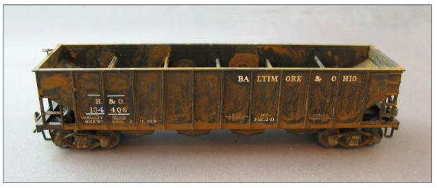
John Schletzer's W-1 from a Bowser PRR H21. The H21s in coke service originally rode on 50-ton archbar trucks, and photos of the B&O's W-1s show many on 50-ton Bettendorf T-sections as John has rendered here.
