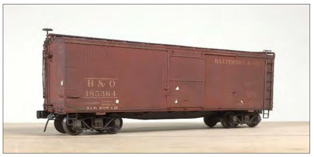
The M-23 car is riding on Tahoe Model Works AC&F arch bar trucks with semi-scale wheelsets. I use Accurail Proto:HO couplers on most of my 1926 equipment.
