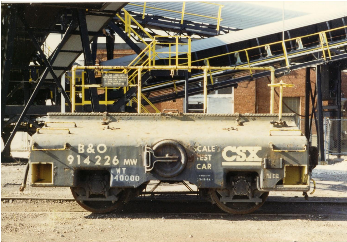
CSX car 914226 , 40,000 lb. car photographed at the Locust Point ore unloader, during the Society's 10/1995 convention. The car was there to test the scale on the ore unloader. To do this it was jacked up and suspended by rods from the scale bin. John Teichmoeller photographs.
