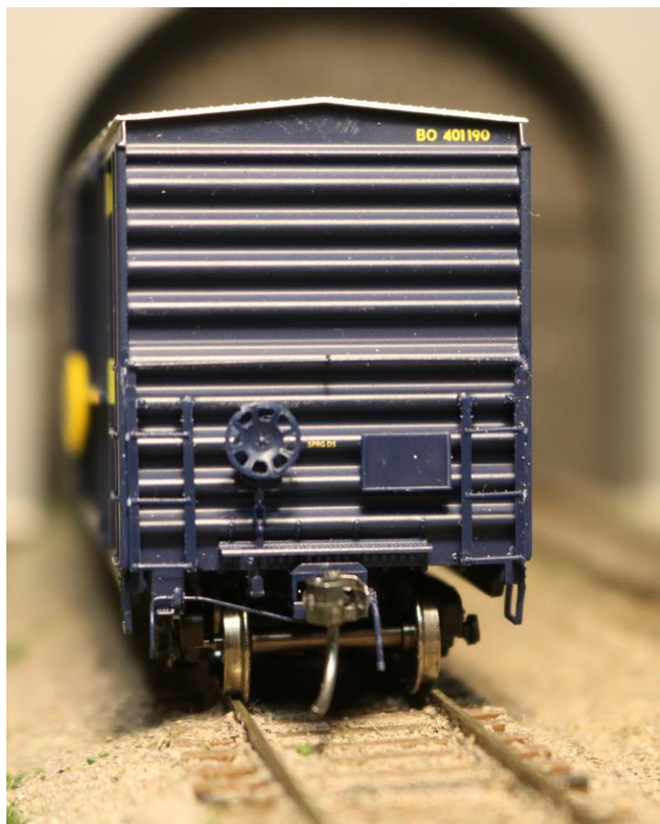
I like the model end. The detail looks good. Note the etched crossover platform and apparent Kadee coupler. A good looking coupler lift bar is installed, as is a simulated air hose.
