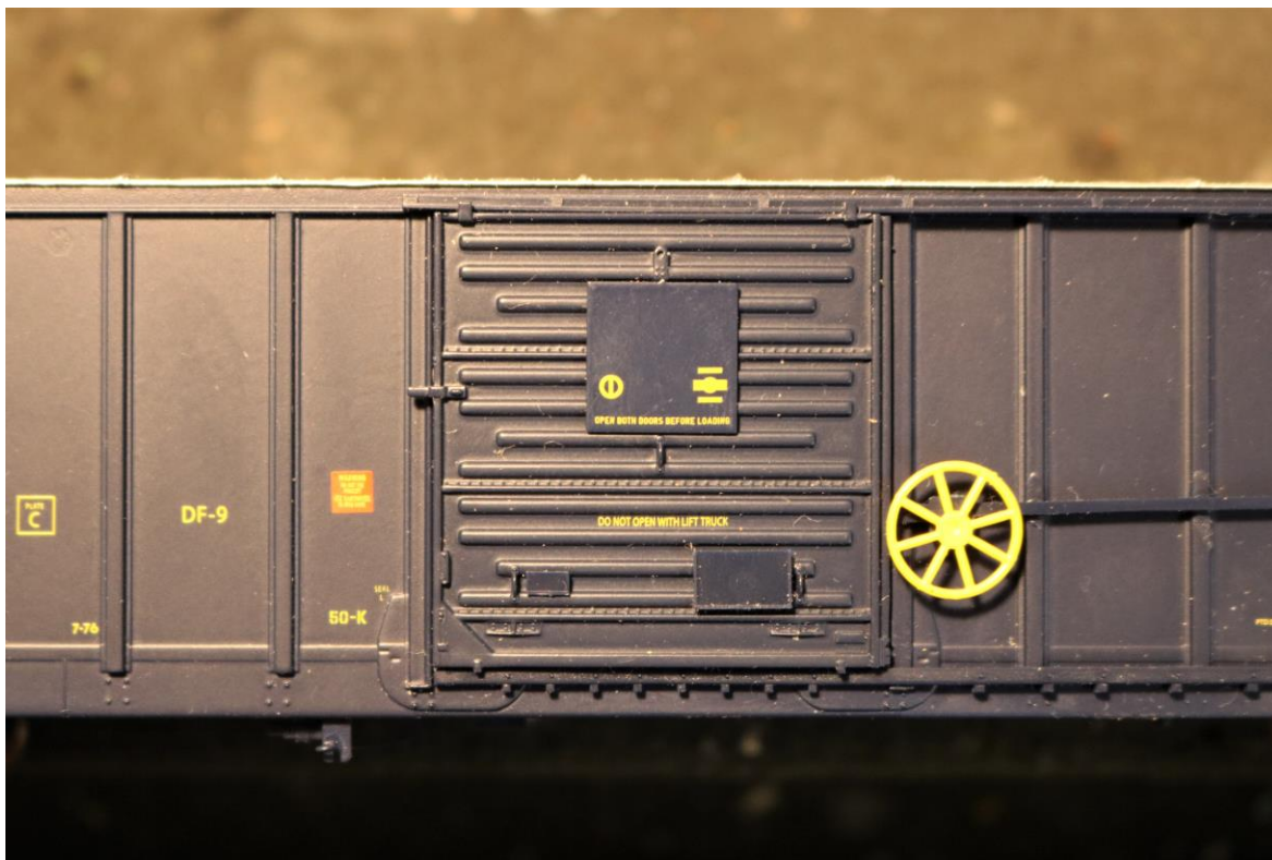
The model, available in at least six road numbers, has a nicely proportioned P-S proprietary door. Note the simulated former NRUC logo plate welded onto the door of a real car.
