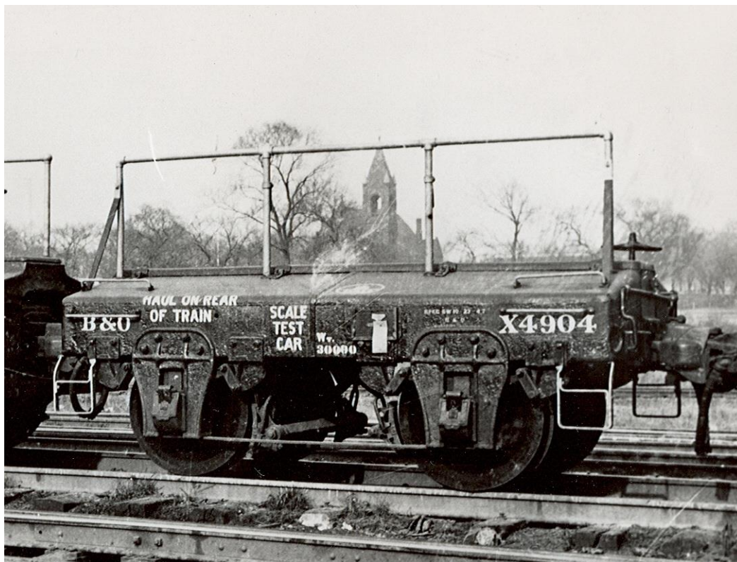
Car X4904, a 30,000 lb. "old style" car with pedestal journal supports. Photographer, date and source unknown.
