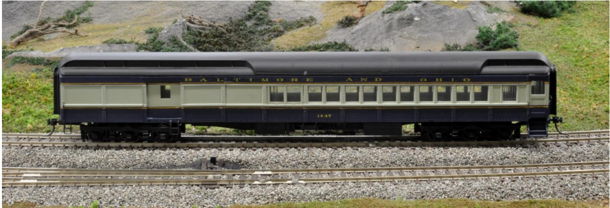
This side of the car, L to R, baggage compartment, coach seating and men's toilet. A/C duct work on this side only.
