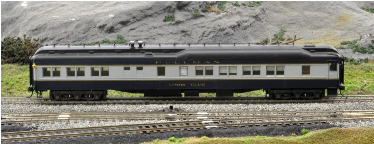
This side of the car, L to R, lounge, buffet, men's lavatory, sleeping sections and hall.
