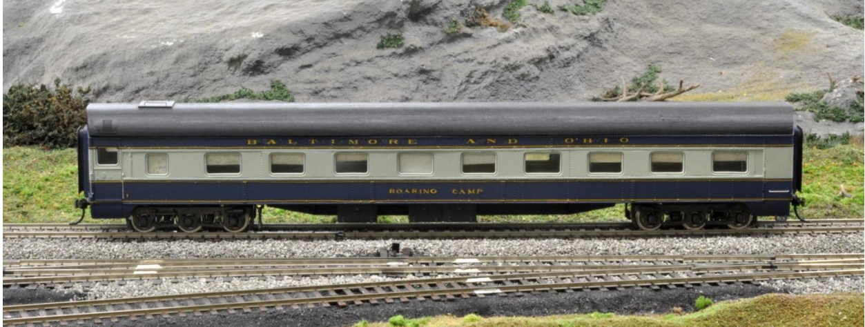
This side of the car, L to R, men's lavatory 1 DR and 8 roomettes.
