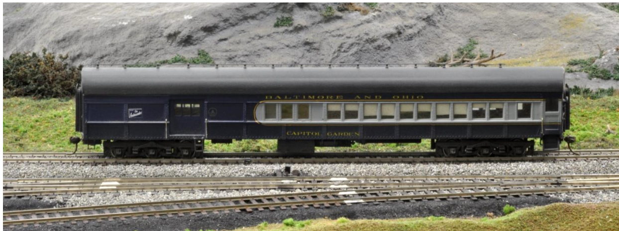
This side of the car, L to R, baggage compartment, dormitory, buffet, lounge and hall.
