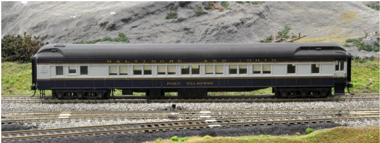
This side of the car, L to R, A/C cooling tower, women's toilet and lavatory, 7 sections and hall across from the men's smoking room, lavatory and toilet. A/C duct work on this side only.
