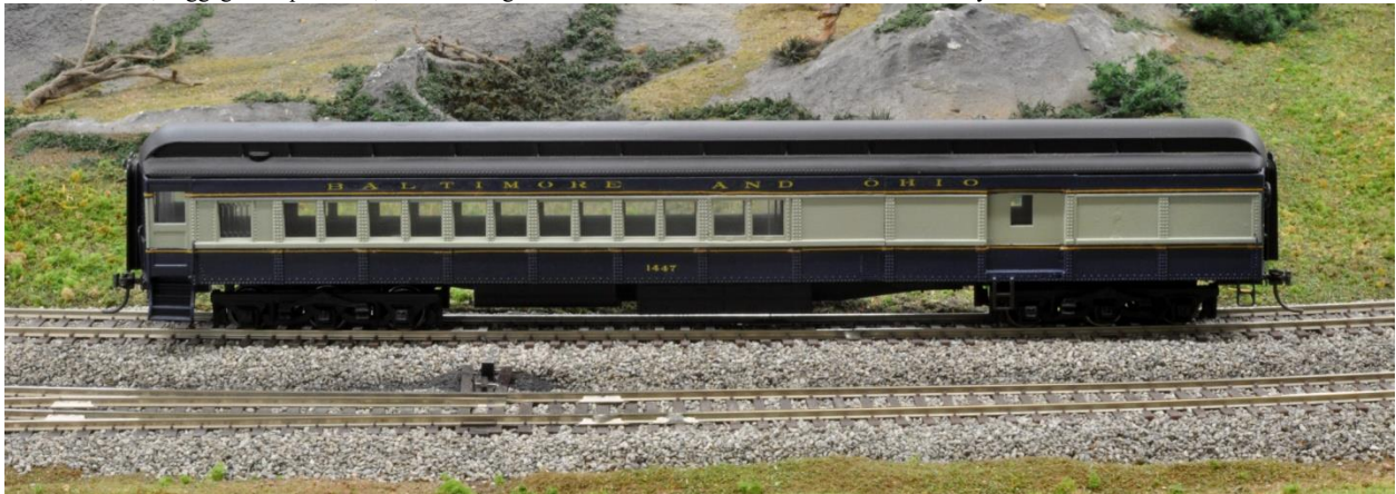
This side of the car, L to R, baggage compartment, coach seating and men's toilet. A/C duct work on this side only.
