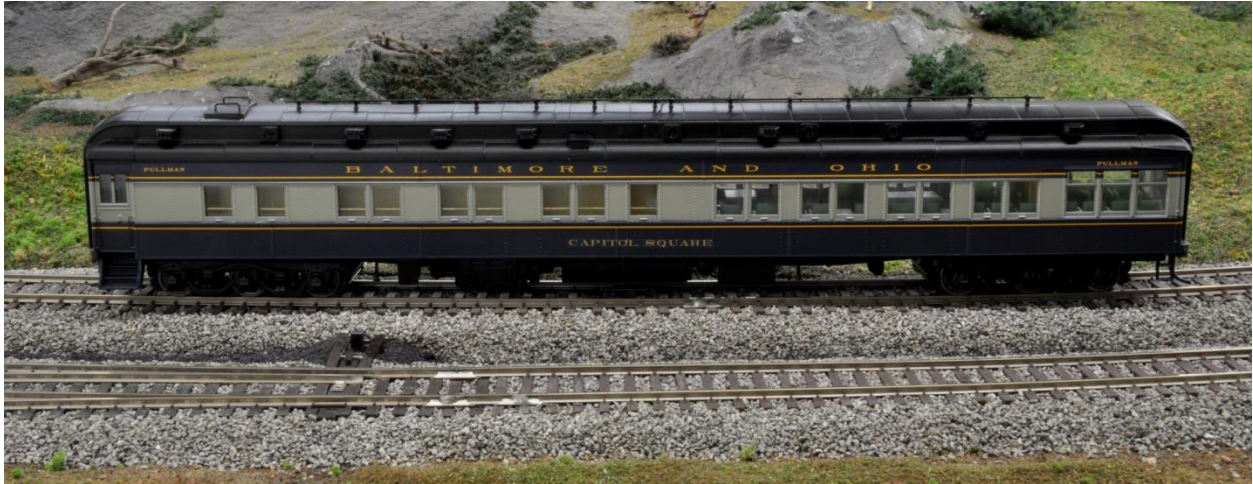
This side of the car, L to R, the hall is on this side of a toilet, 2 compartments, 1 drawing room, 1 compartment and the buffet, lounge and sun room.
