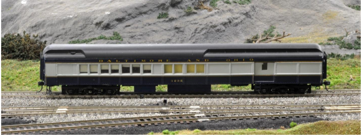
This side of the car, from L to R, storage locker, A/C compartment, lounge, hall across from the buffet and dormitory and the baggage compartment.
