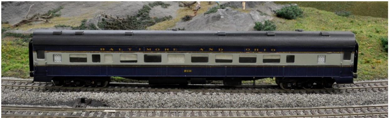
This side of the car, from L to R, Drawing Room lavatory and Drawing Room, 26 seat parlor seating and men's lavatory.
