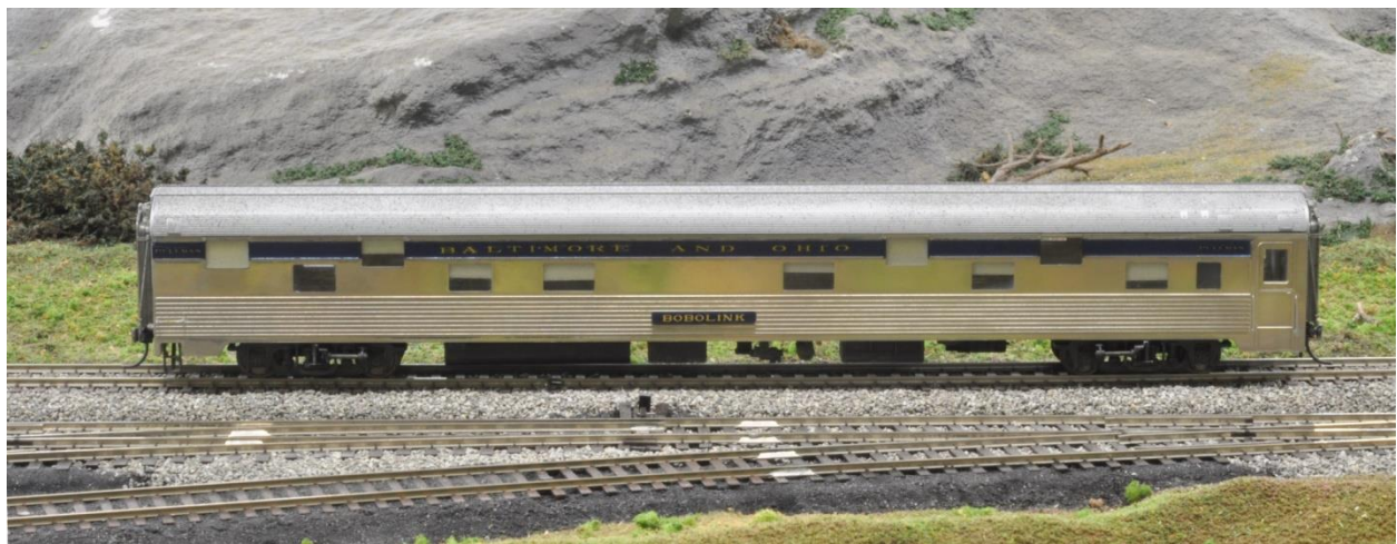
This side of the car, L to R, 4 roomettes, hall across from 4 bedrooms, 4 roomettes and a lavatory.
