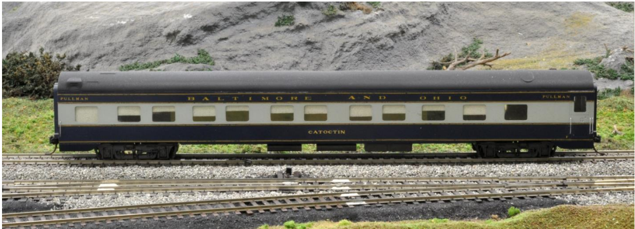
This side of the car, L to R, 3 roomettes, 6 bedrooms and 3 roomettes.
