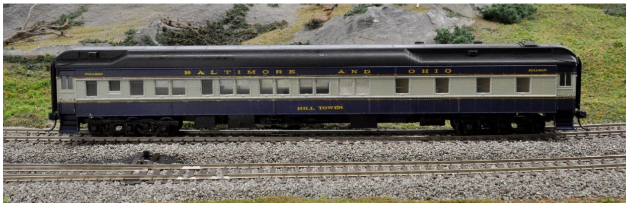
This side of the car, from L to R, men's lavatory and smoking room, 1 drawing room, 4 sections and the hall across from the 3 double BR and the women's lavatory.
