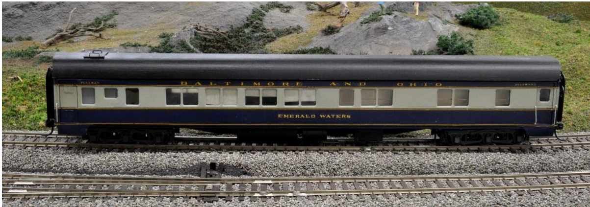
This side of the car from L to R, the A/C cooling tower, men’s lavatory, 4 sections and the hall across from the 4 Double B.R. and the Womens lavatory.
