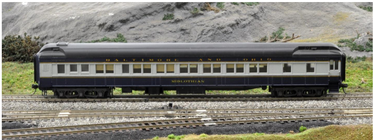
This side of the car, L to R, A/C cooling tower, women's toilet and lavatory, 1 DR, 6 sections and the hall across from the men's smoking room, lavatory and toilet. A/C duct work on this side only.
