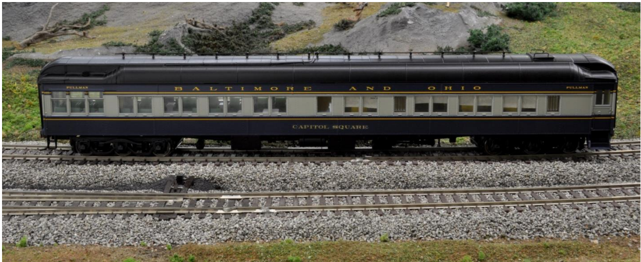
This side of the car, L to R, sunroom, lounge, buffet, 1 compartment, 1 DR, 2 compartments and a toilet.
