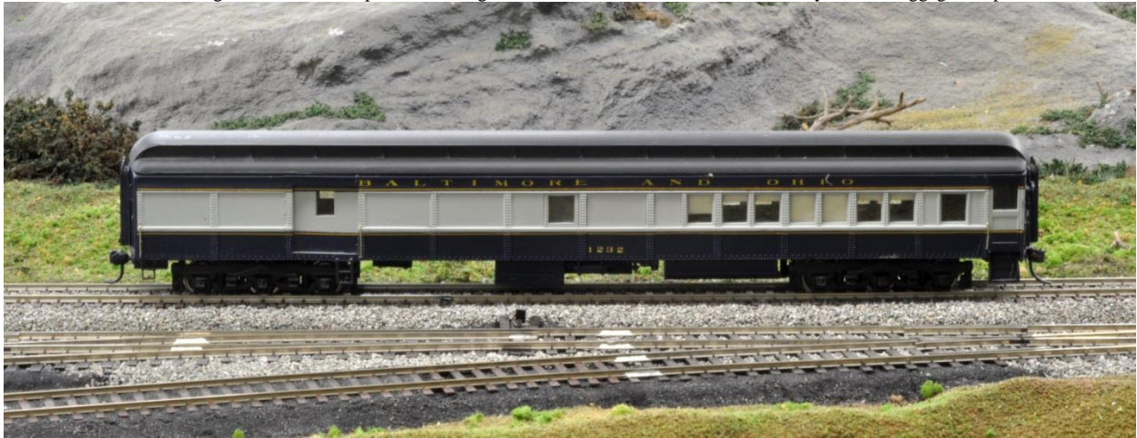
This side of the car, from L to R, storage locker, A/C compartment, lounge, hall across from the buffet and dormitory and the baggage compartment.
