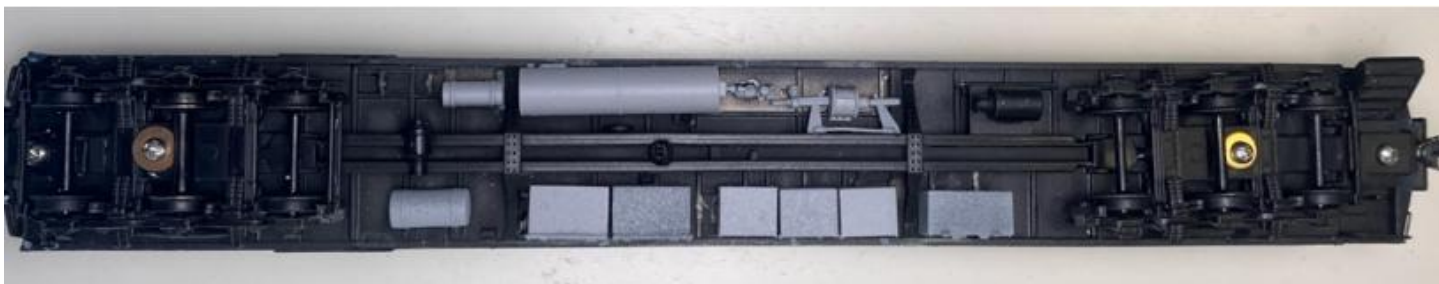
(Image 11 - Baggage end to the left, Lounge end and steps to right. The boxes are on the corridor side of the car, water tank and brake cylinder on galley/dorm side of car.)
