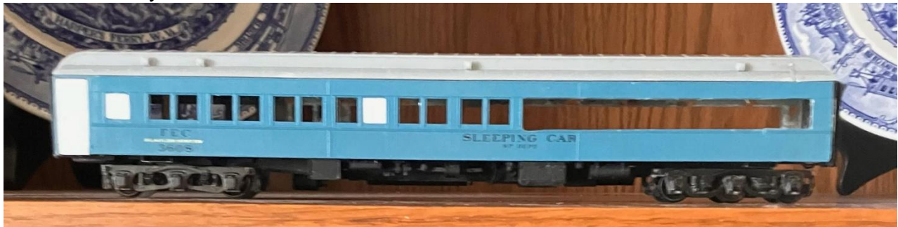
(Image 6, side A: (corridor side) Going right to left, cut out the lavatory window nearest the right end and the next four pairs of double windows for the baggage end. Later we will blank two windows and the door with styrene sheet.)
