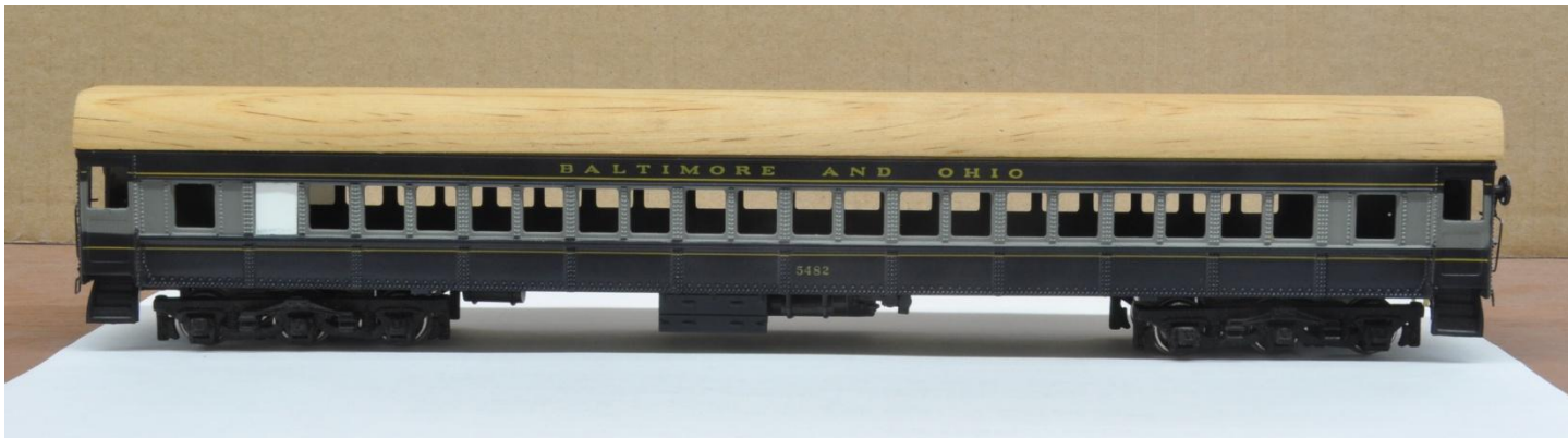
(A window is blanked out for an electrical compartment.)
