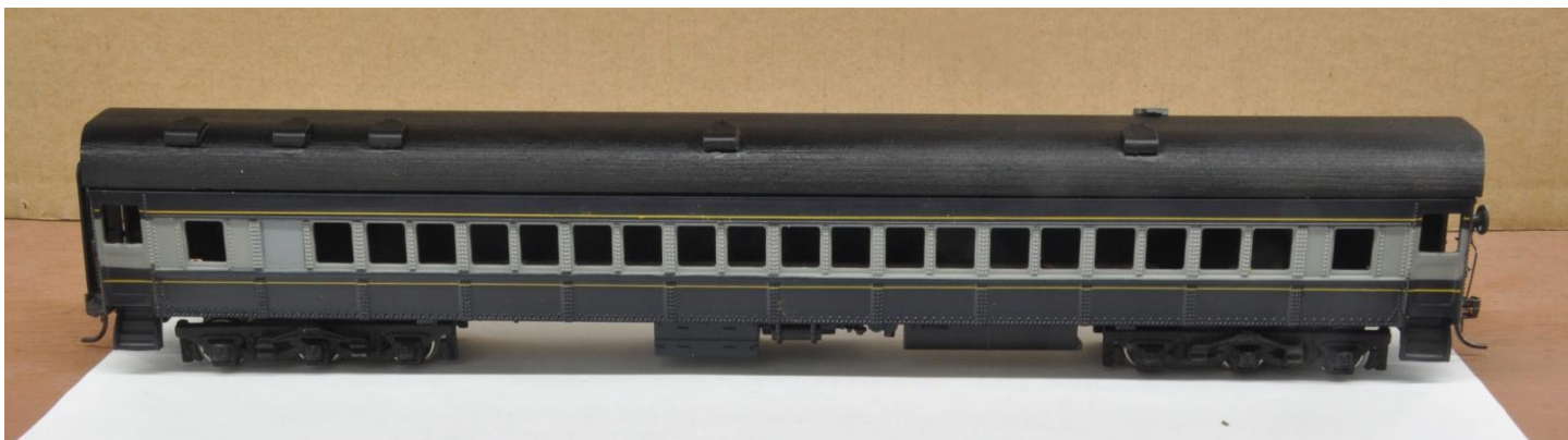
(BCW roof vents have been added and the roof painted. The NERS Pullman 145-gal water tank has been assembled, painted and installed, and blanked out window has been painted gray).
