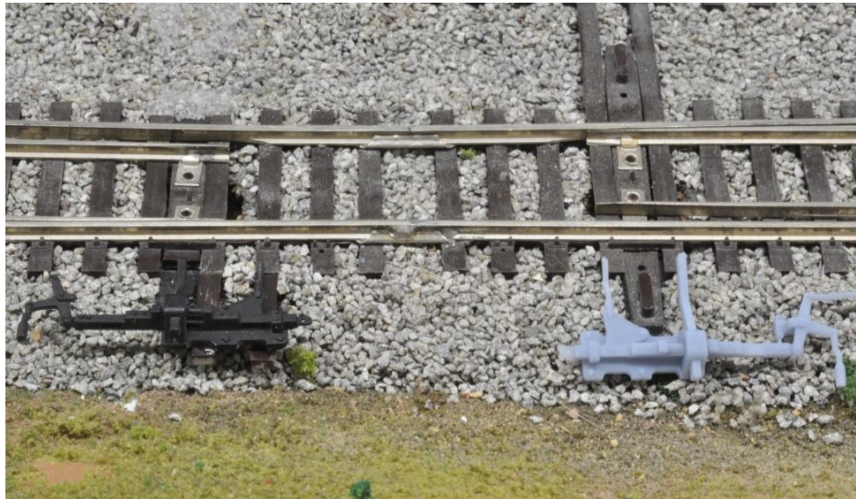
(Turnouts and switch machines! My layout is populated with Shinohara turnouts, But I believe that all commercial turnouts need to be modified for correct placement of Armstrong switch machines. Close inspection reveals that switch stand tie extensions needed to be moved from one side to the other and that the pair needed to be moved one tie forward for proper seating of the switch machine. It is also necessary to remove the excess throw bar material.)
