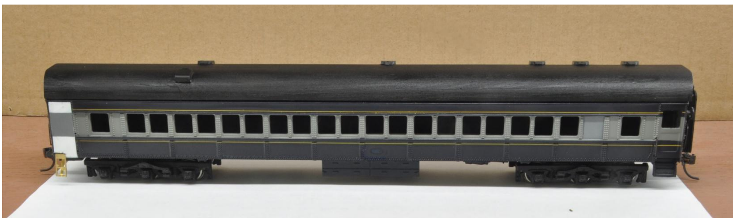
(Lettering and numbers have been removed, Kadee couplers installed, blanked out window at the right and vestibule pillow locker at the left have been painted gray. One diaphragm at the right has been installed. The other diaphragm will be installed after the enclosed vestibule door receives a coat of blue paint. A note: only the blanked-out panels were masked and painted. That is how closely the Floquil color matched the Bachmann model.)
