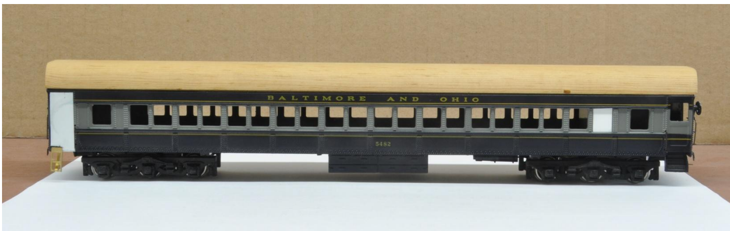
(At the left, a vestibule door has been blanked out and this half of the vestibule is now a pillow locker. A stirrup step replaces the stationary vestibule steps. The blanked-out window at the right is the A/C compartment.)
