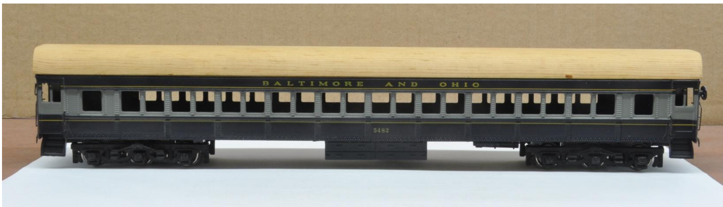
(A new betterment roof, no rubber diaphragms and the PRR water tanks are gone as are the couplers. Even in this state the car looks 100% better.)
