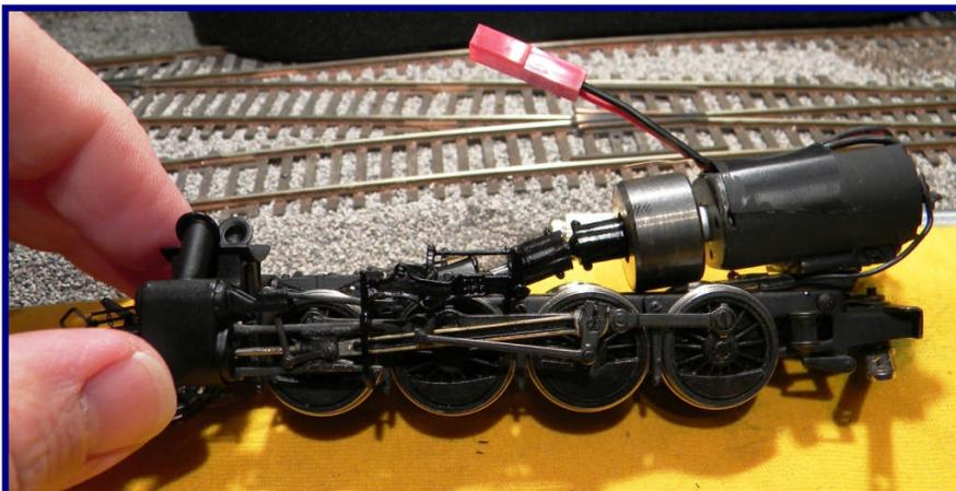
I made a small motor mounting plate that could be screwed to the original motor saddle. In this way I can attach the positive wire to the frame, at the same time, mounting the motor with clear silicone gel. This worked out well. I soldered a micro-plug to the motor, in order to connect the headlight wires. This makes future shell removal less difficult. Those of you who have moved to the dark side (DCC) will do this differently.
