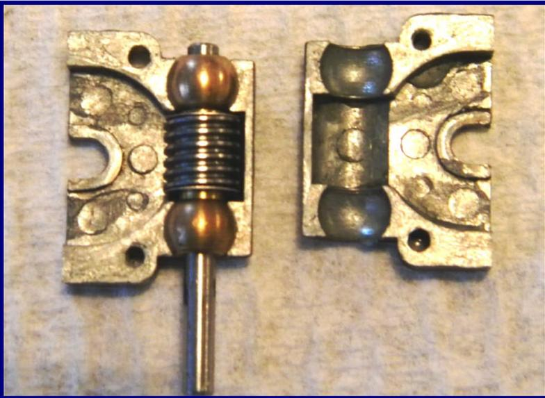
Gearbox cleaned and additional thrust washers installed. In this photo the thrust washers are added on either side of the worm. The new washers were ultimately mounted outside the stock thrust washers.
