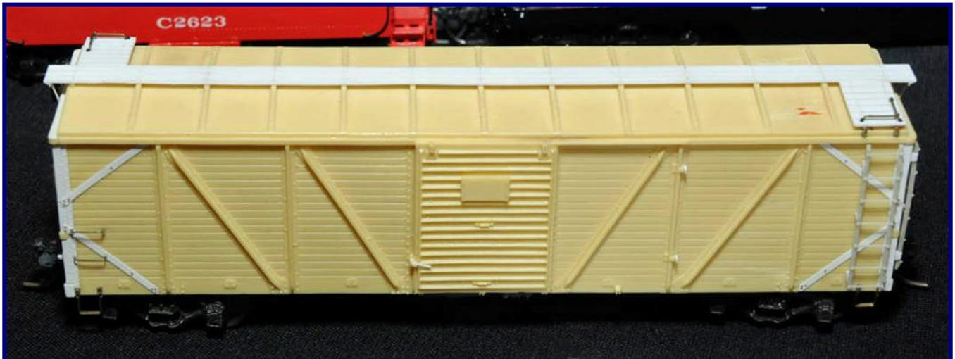
WAG (ex-B&M) XM-1 single sheathed boxcar, upgraded Yankee Clipper (Funaro & Camerlengo) HO scale model by Byron Rose, Cocoa Beach 2014.
