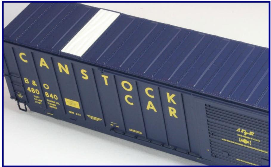
There are a lot of small details that I like about the design of this model. They included a separate door track as other manufacturers have offered recently, since that has become the new "standard" for HO models. They used metal screws to secure the weight inside the car so the glue doesn't come loose, and they used wire instead of plastic for the piping between brake components to make it more durable.
