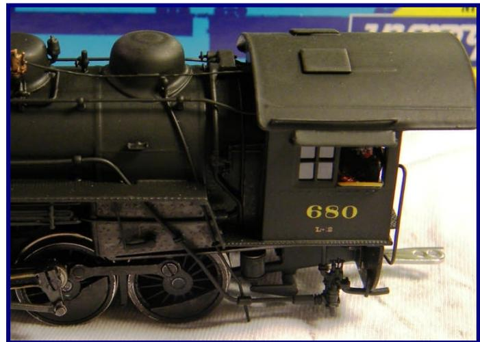
The lift bar and coupler head are connected with fine blackened chain. The windows are glazed, with the "glass" held in place with white glue. Someday I want to try using microscope cover glass (slide covers).
