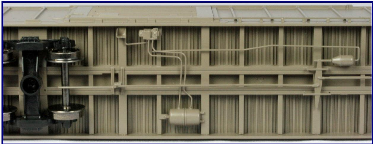
Corrected Brake Details on Second Test Sample
