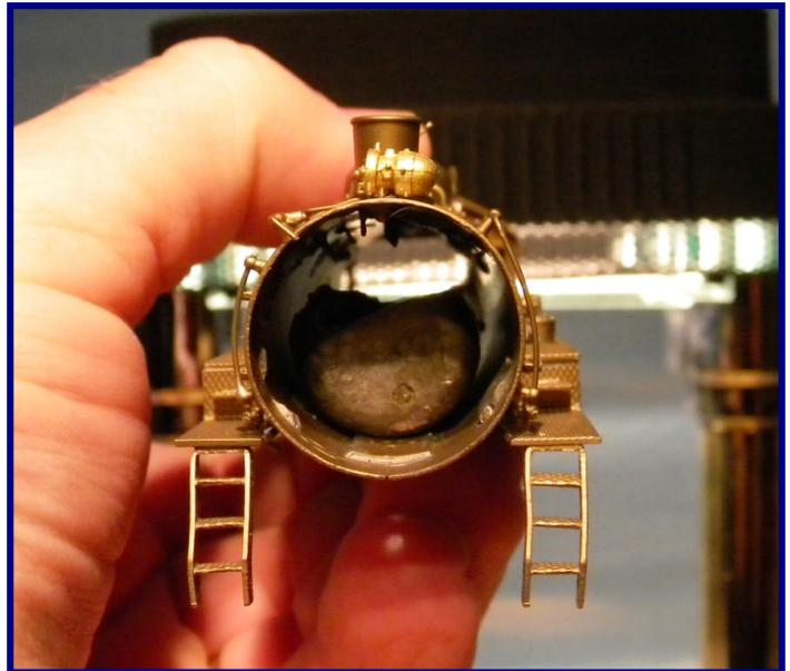
Boiler weight is filed down to allow plugs and wires to pass to the headlight. Locomotive still has plenty of weight for pulling.
