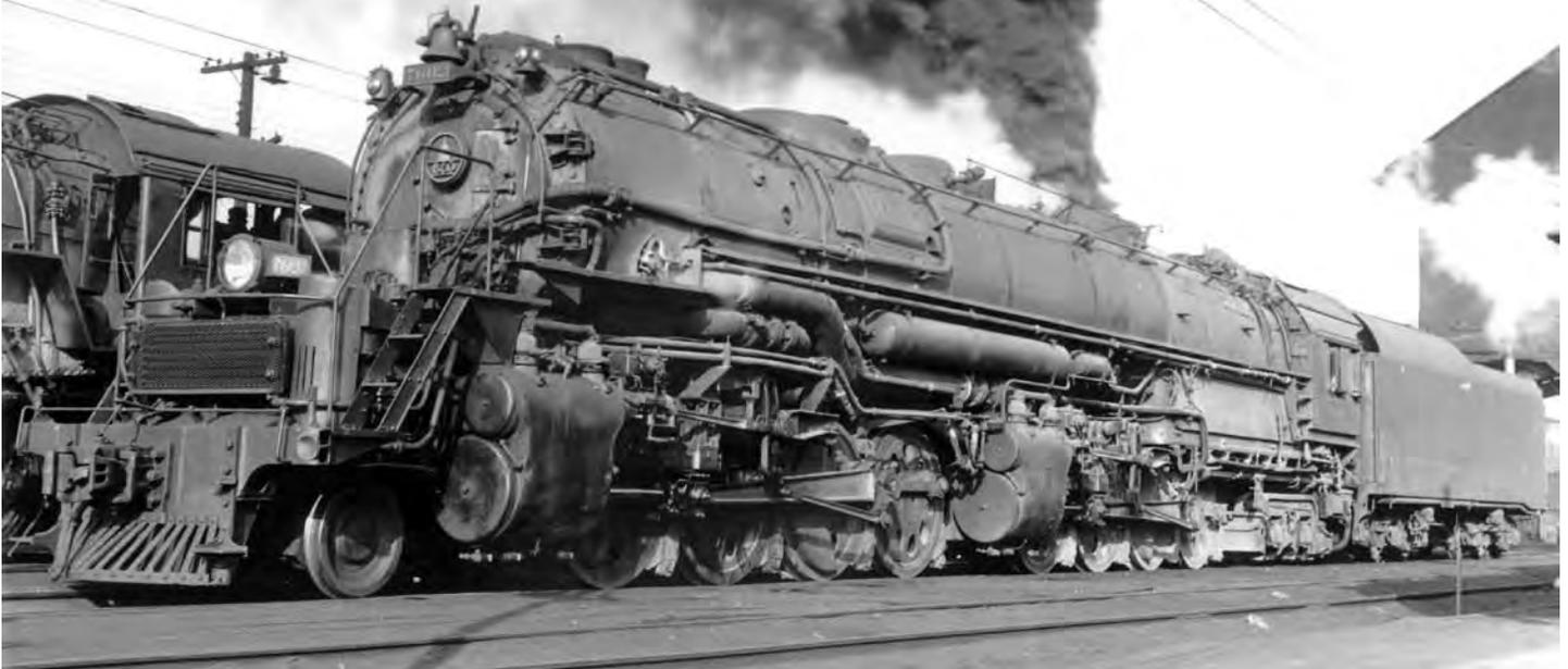
Locomotive 7602 at Cumberland Engine Terminal, July 8, 1948. Notice that the engine has the original globe marker lamps and the location of sandbox filler hatches. The check valve has been relocated from the side of the boiler to the top.
